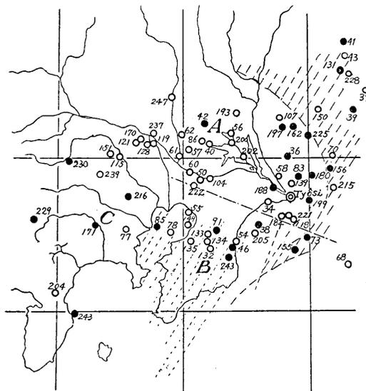
Fig. 1 (c). Distribution of initial motion observed at Tyôsi.
