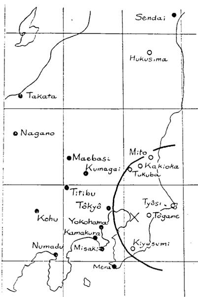
Fig. 4. Distribution of initial motion of earthquake occurred on May 21, 1928.
