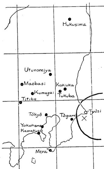
Fig. 2 (c). Distribution of initial motion of the earthq. occurred on May 1, 1930.
