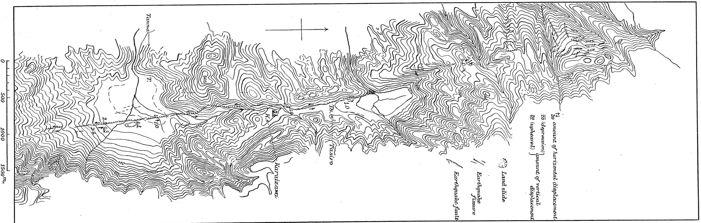
Fig. 12. Map showing the distribution of ground disturbances along the Tanna fault zone (Part I. North part.)
