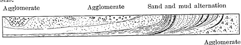
Fig. 7. Schematic geologic sketch of the tunnel wall between stations 6950 ft. and 7350 ft. from the western mouth.
