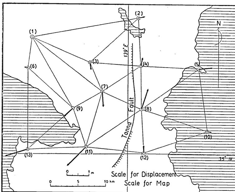
Fig. 15. Map showing the displacement of triangulation point in Northern Idu (after C. Tsuboi).
