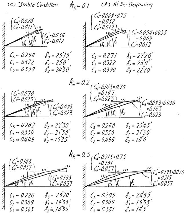
Fig. 15-II. Variation of earth pressure against a vertical wall during vibration.
