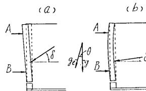
Fig. 18. Yielding of the wall under elastic supports (a) and solid supports (b).
