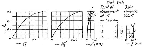
Fig. 9. An example of the results of tests under stable condition. (Solid supports;  $b=39.6$ ,  $h=30$ ,  $t=1.5$  cm)
