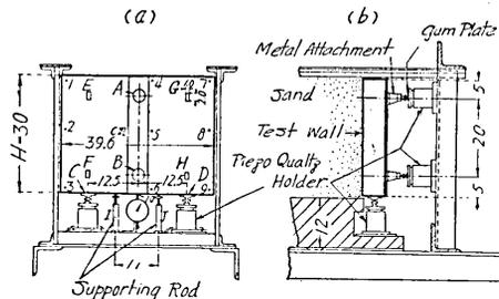
Fig. 2. Test wall installed for measurement.
