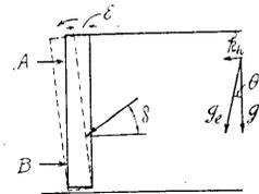
Fig. 4. Yielding of wall under elastic supports.
