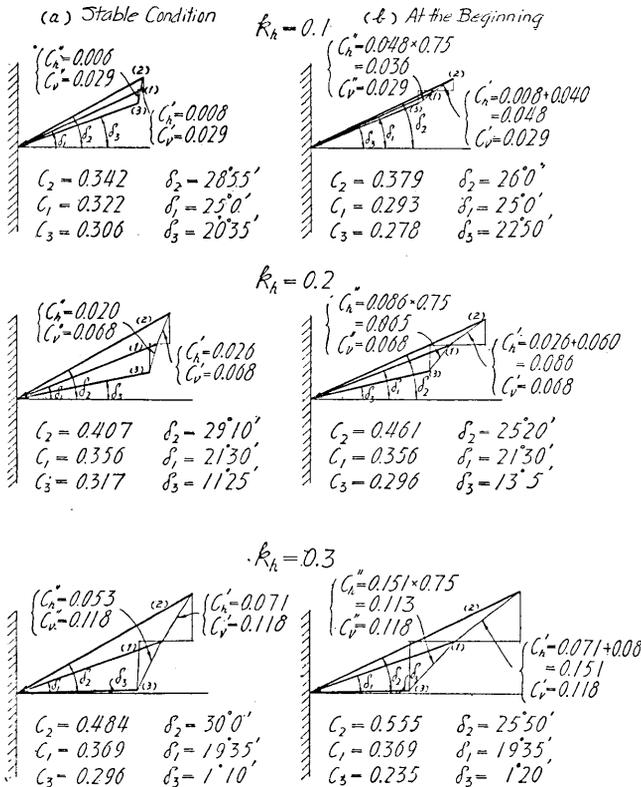
Fig. 15-I. Variation of earth pressure against a vertical wall during vibration.
