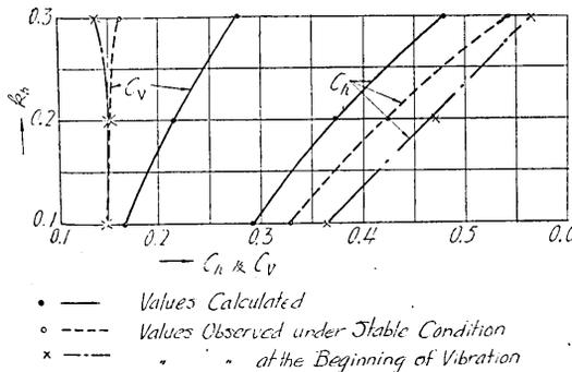
Fig. 17. Comparison of the values observed with calculated. (Solid supports)
