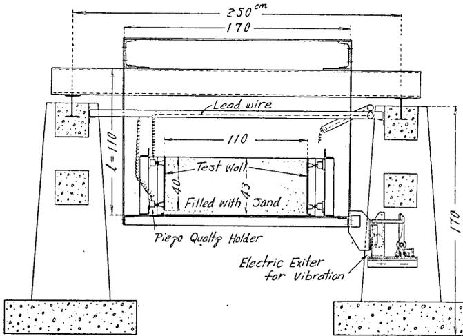
Fig. 1. Test box with the supports.
