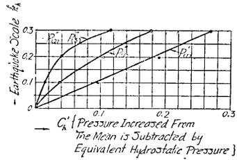
Fig. 6. Variation of horizontal pressure at the beginning of vibration under elastic supports.
