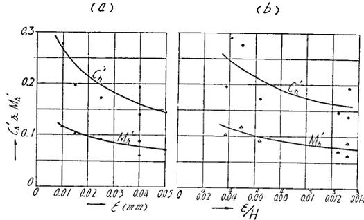
Fig. 10. Relation between  $\epsilon$  and  $C_h'$  etc. under stable condition. (Solid supports;  $k_h=0.3$ )
