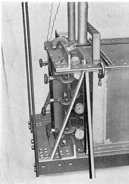
(2) Measuring apparatus of the deflection of the wall.
