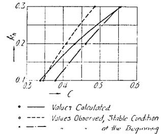
Fig. 16. Comparison of the values observed with calculated. (Elastic supports)
