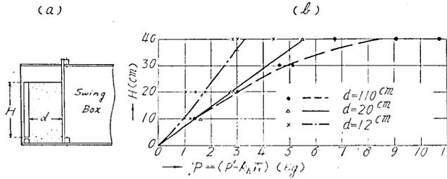
Fig. 14. Effect of  $d$  on the pressure.
