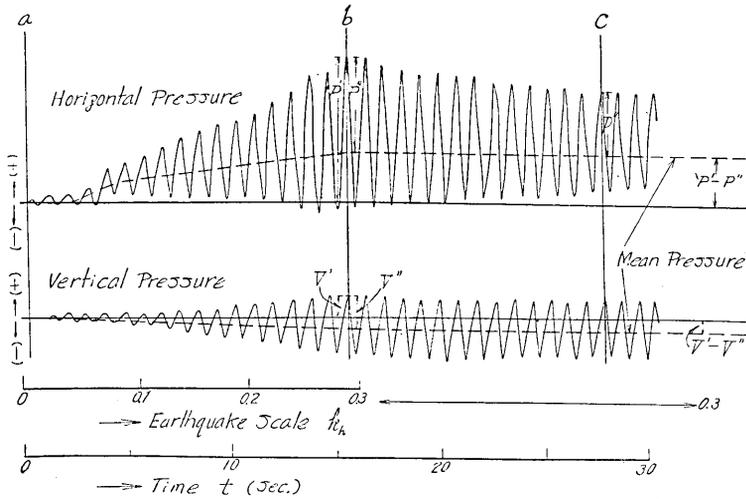
Fig. 5. Typical record of pressure at the beginning of vibration.
