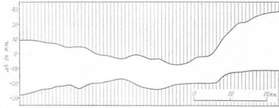
Fig. 18. Overrapping Means of the Change of Height of the Bench Marks on the Route from Ootu to Miyake during 1918-1888 (Upper Curve) and 1927-1918 (Lower Curve).
