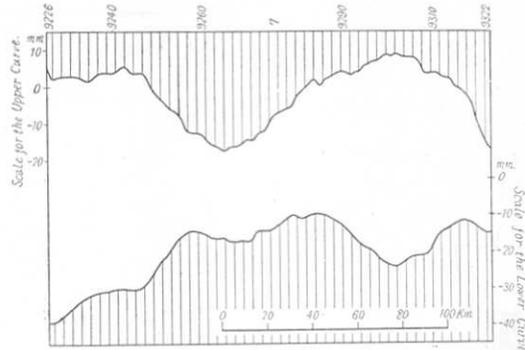
Fig. 13. Overrapping Means of the Change of Height of the Bench Marks on the Route around Noto Peninsula during 1917-1900 (Upper Curve) and 1928-1917 (Lower Curve)
