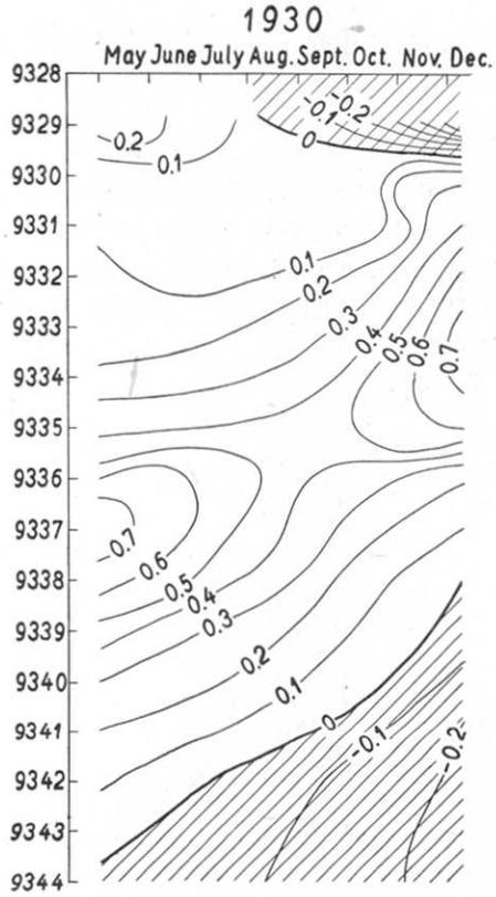
Fig. 29. Daily Vertical Velocities of Different Bench Marks in the Ito District in mm.
