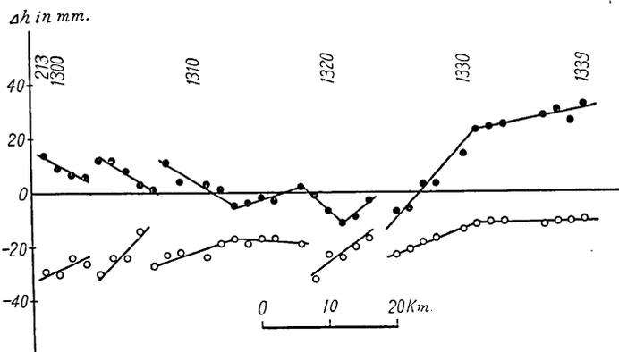
Fig. 17. Change of Height of the Bench Marks on the Route from Ootu to Miyake.
