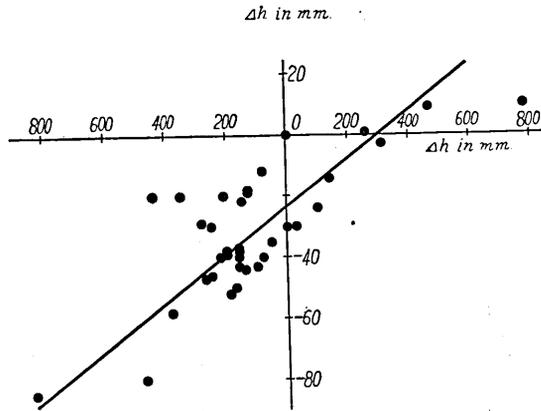
Fig. 2. Correlation Diagram for the Measured Change of Height of the Bench Marks in the Tango District at the Time of (Abscissa) and After (Ordinate) the Tango Earthquake of 1927.
