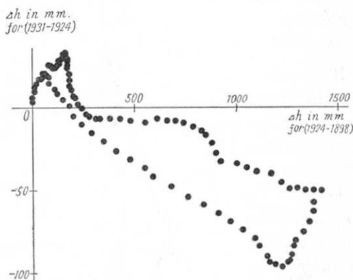
Fig. 11. Correlation Diagram for the Overrapping Means of the Change of Height of the Bench Marks on the Route around Boso Peninsula at the Time of (Abscissa) and After (Ordinate) the Kwantô Earthquake of 1923.
