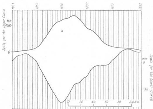
Fig. 10. Overrapping Means of the Change of Height of the Bench Marks on the Route around Boso Peninsula at the Time of (Upper Curve) and After (Lower Curve) the Kwantô Earthquake of 1923.
