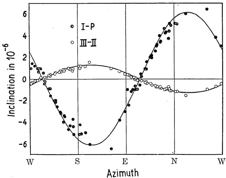
Fig. 26. Sine-Curves Indicating the Tilting of a Land Block in the Sakurazima District.
