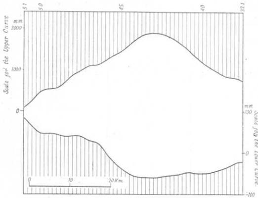
Fig. 8. Overrapping Means of the Change of Height of the Bench Marks on the Route from Hudisawa to Atami at the Time of (Upper Curve) and After (Lower Curve) the Kwantô Earthquake of 1923.
