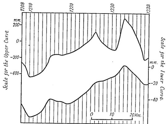
Fig. 1. Overlapping Means of the Change of Height of the Bench Marks in the Tango District at the Time of (Upper Curve) and After (Lower Curve) the Tango Earthquake of 1927.
