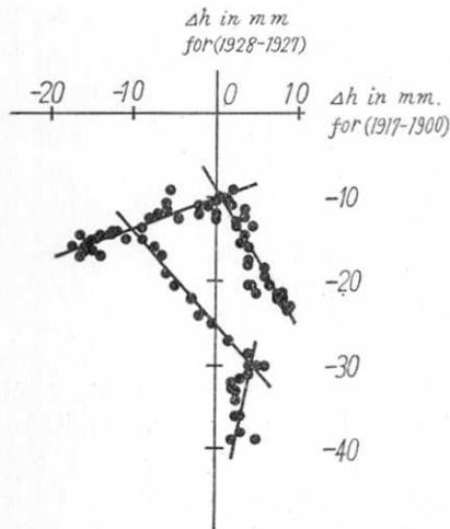
Fig. 15. Correlation Diagram for the Overlapping Means of the Change of Height of the Bench Marks on the Route around Noto Peninsula during 1917-1900 (Abscissa) and 1928-1917 (Ordinate).
