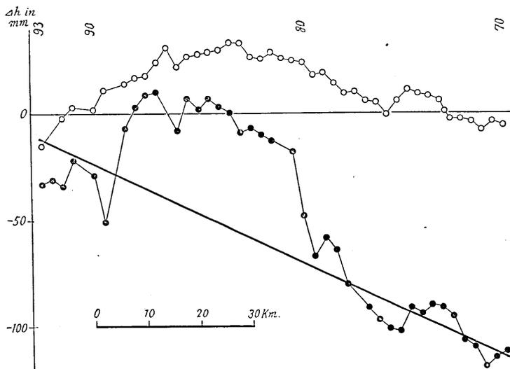
Fig. 5. Change of Height of the Bench Marks on the Route from Okitu to Kôhu.
