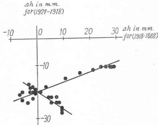
Fig. 19. Correlation Diagram for the Overrapping Means of the Change of Height of the Bench Marks on the Route from Ootu to Miyake during 1918-1888 (Abcissa) and 1927-1918 (Ordinate).
