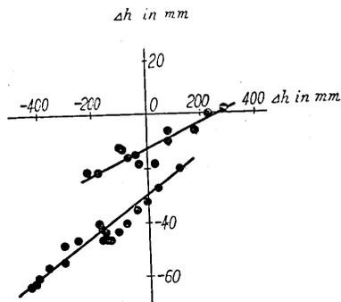
Fig. 3. Correlation Diagram for the Overrapping Means of the Change of Height of the Bench Marks in the Tango District at the Time of (Abscissa) and After (Ordinate) the Tango Earthquake of 1927.
