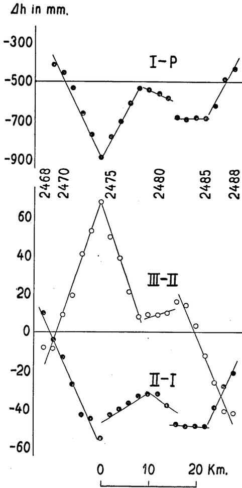
Fig. 21. Change of Height of the Bench Marks in the Sakurazima District Before and After the Eruption of 1914.
