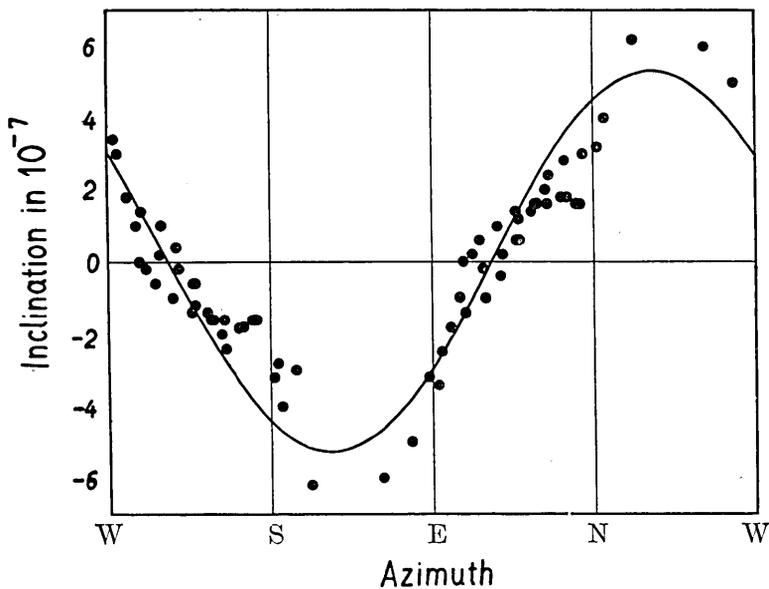
Fig. 27. Sine-Curve indicating the Tilting of a Land Block in the Sakurazima District during (1915-1914).
