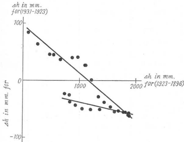
Fig. 9. Correlation Diagram for the Overrapping Means of the Change of Height of the Bench Marks on the Route from Hudisawa to Atami at the Time of (Abscissa) and After (Ordinate) the Kwantô Earthquake of 1923.
