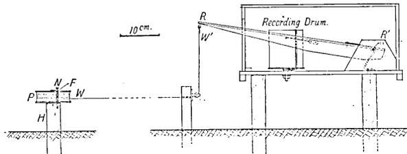
Fig. 2. Side-view of the self-recording instrument.
