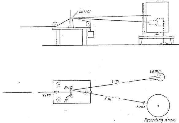
Fig. 7. Photographic recording apparatus for landslide observation. Upper = elevation, lower = plan.
