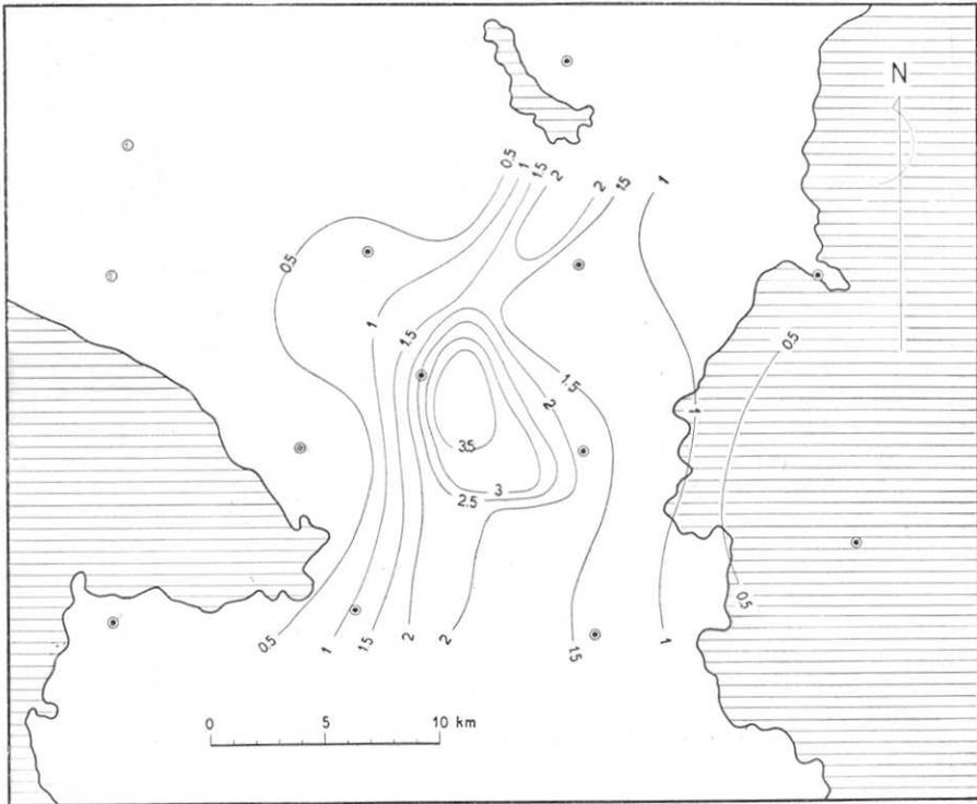
Fig. 10. Lines of Equal Maximum Shear in  $10^{-5}$ .
