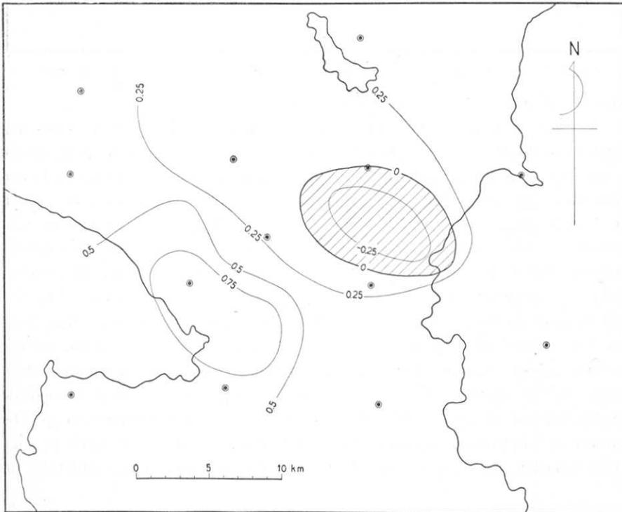
Fig. 5. Lines of Equal Northward Gradient of Eastward Displacement in  $10^{-5}$ .
