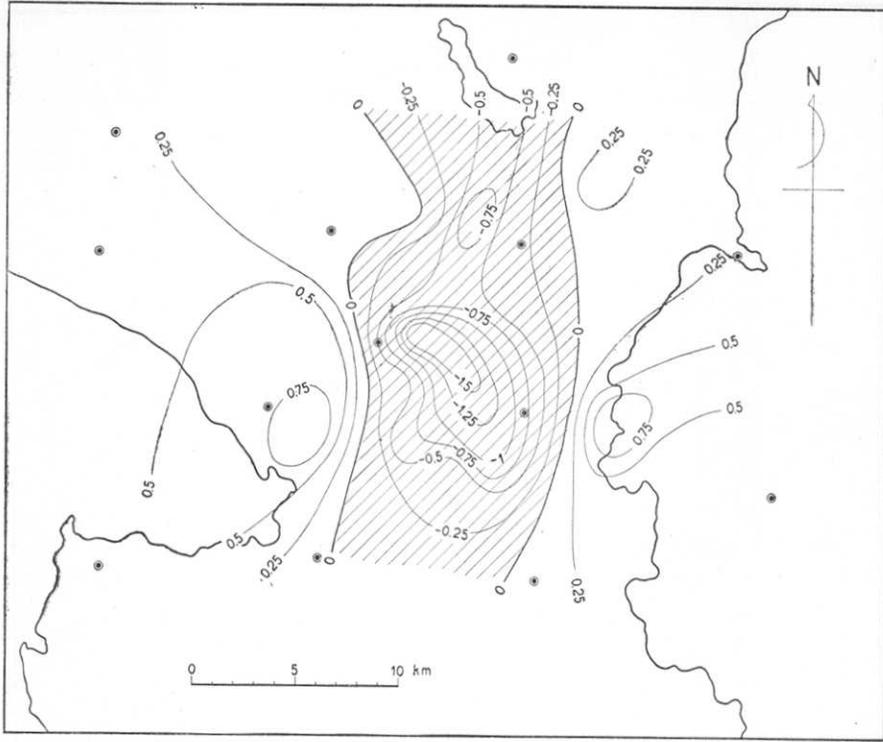
Fig. 8. Lines of Equal Rotation  $\frac{1}{2} \left( \frac{\partial u}{\partial y} - \frac{\partial v}{\partial x} \right)$  in  $10^{-5}$ .
