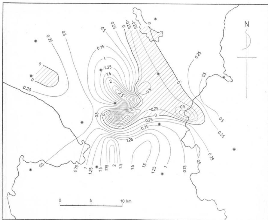
Fig. 7. Lines of Equal Dilatation  $\left(\frac{\partial u}{\partial x} + \frac{\partial v}{\partial y}\right)$  in  $10^{-5}$ .
