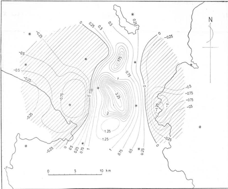
Fig. 4. Lines of Equal Eastward Gradient of Northward Displacement in  $10^{-5}$ .
