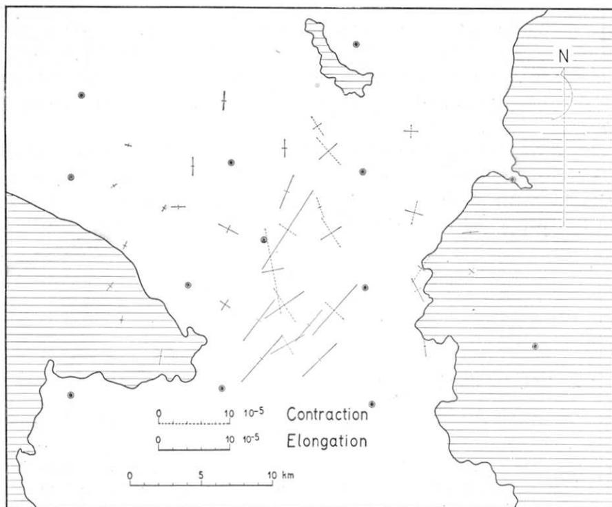
Fig. 11. Principal Axes of Strain Ellipses.
