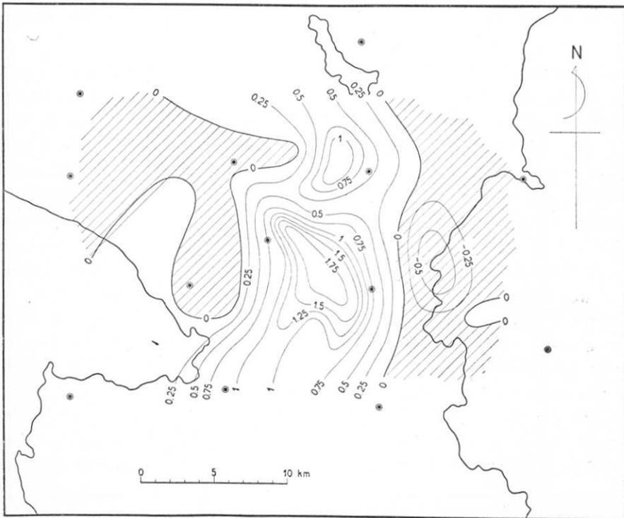
Fig. 9. Lines of Equal Shear  $\frac{1}{2} \left( \frac{\partial u}{\partial y} + \frac{\partial v}{\partial x} \right)$  in  $10^{-5}$ .
