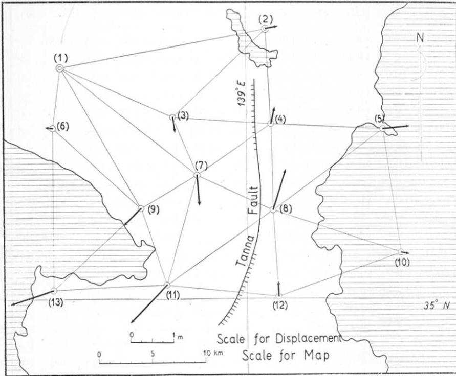
Fig. 2. Horizontal Displacements of the Triangulation Points in Idu Peninsula.
