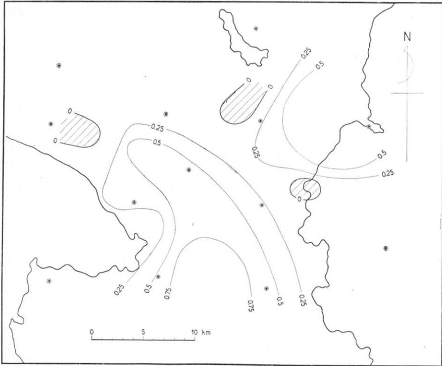
Fig. 3. Lines of Equal Eastward Gradient of Eastward Displacement in  $10^{-5}$ .
