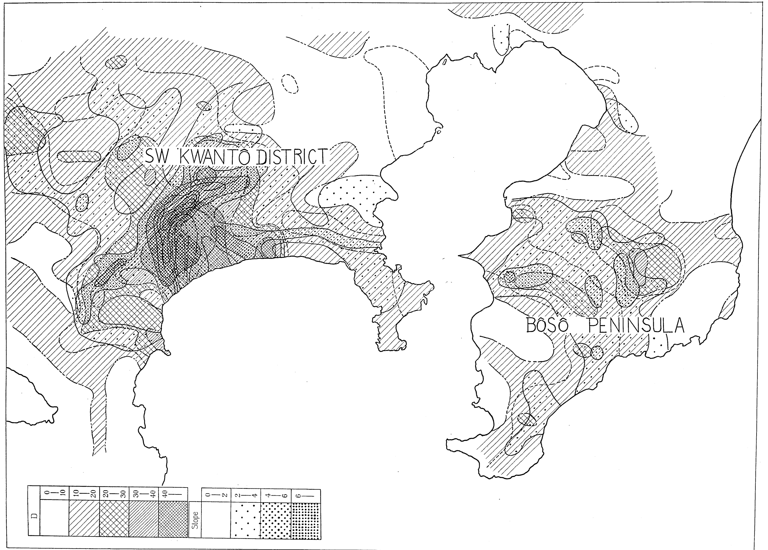
Fig. 3. Distribution of D and Slope of Vertical Displacements.
