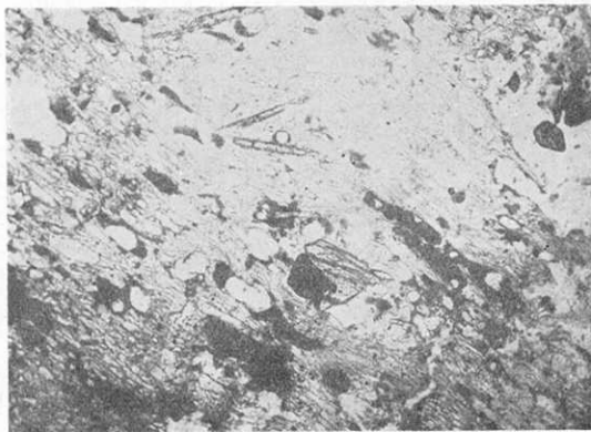
Fig. 3. Microphotograph of pyroxene-andesite scoria ×40.
