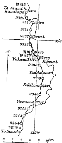
線路圖 (數字ハ水準點番號ヲ示ス) Map of route. (Figures show the numbers of bench marks.)
