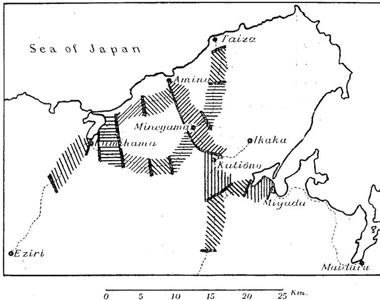
of these lines corresponding to a unit of structure of the ground. The bench marks lying on one and the same unit are rigidly connected to each other, being only subjected to the common tilting, upheaval, depression, etc., of the unit as a whole. In Fig. 3, the inclination of some of the structural units is seen to be inverted in sense for different epochs of the levellings. Each structural unit must have been able to move comparatively easily at least after the great earthquake.
