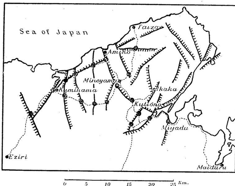
The levelling routes cross with several of these lines at the points marked by black dots as shown in Fig. 5. When the positions of these points are compared with those of boundary lines between the structural units in Fig. 4, a very close coincidence is found to exist between them.
