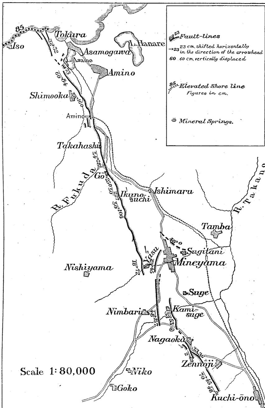
Fig. 4. The vertical and horizontal displacements of the land to the west of each rift of the Gōmura fault.
