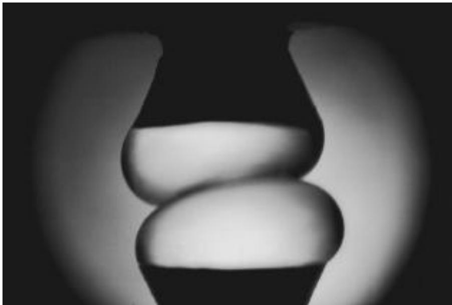
Fig. 4.3 Non-coalescence of two 5 cSt silicone oil drops. The rods have a diameter of 3.00mm. Pressing against one another clearly deforms the interfaces. [22]
