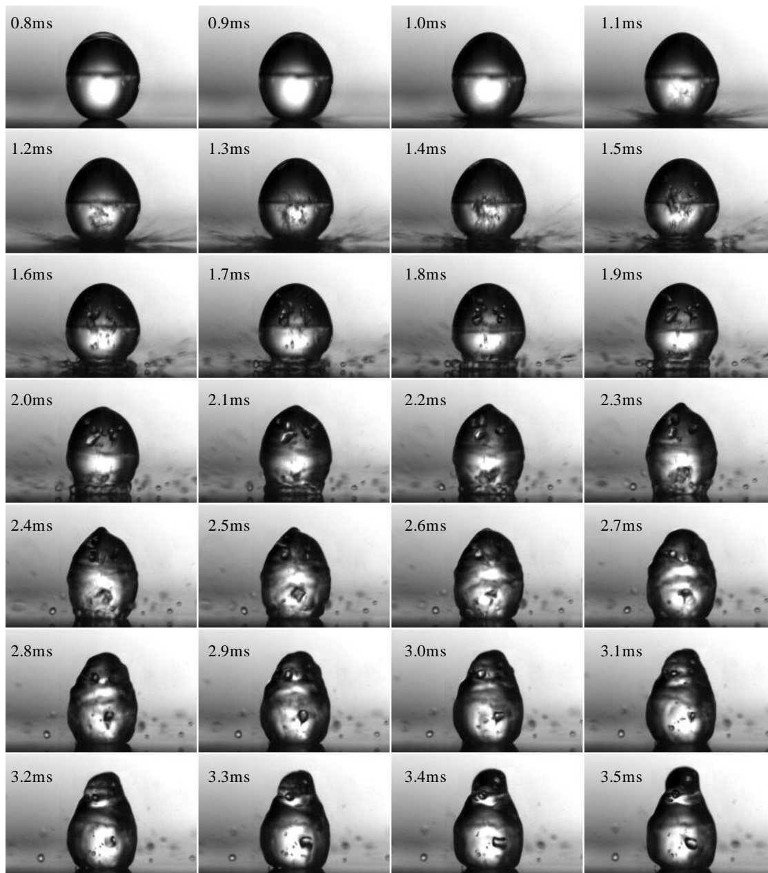
Fig. 4 Time sequential images of the droplet during jet ejection. The collided surface was heated copperplate. These images are the behavior of droplet during first collision. The surface temperature of the plate was 311°C. The first collision velocity of the droplet was 311°C.
