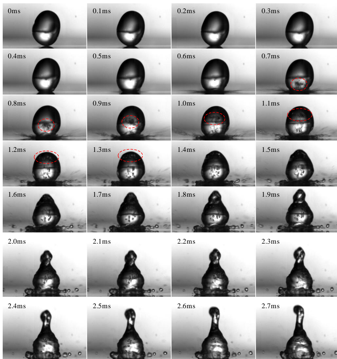
Fig. 3 Time sequential images of the droplet during jet ejection. The collided surface was heated copperplate. These images are the behavior of droplet during second collision. The surface temperature of the plate was 313°C. The first collision velocity of the droplet was 0.34m/s. The dotted red line circle shows the movement of the vapor that was generated at the the bottom interface of the droplet.
