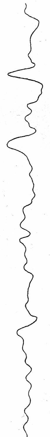
Transverse Motion. Locomotive N o 85 Dubs. Scale 1 \frac{in}{10 min} Speed 35 \frac{mi}{hr}
