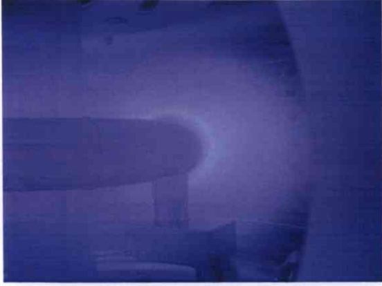
Figure 2.17: A photograph of a plasma with the simple dipole configuration.
