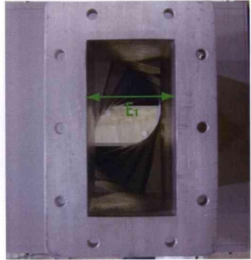
Figure 4.2: Waveguide for X-mode injection.
