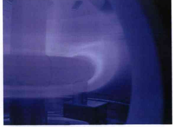
Figure 2.18: A photograph of a plasma with the separatrix configuration.
