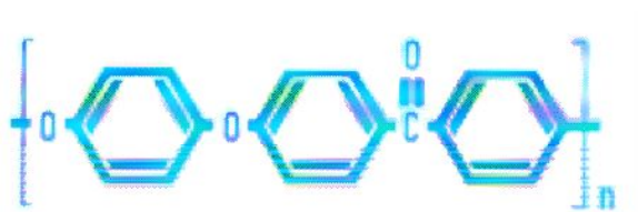
Fig. 4.1 PEEK monomer.
