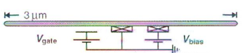
Fig. 1.14 The electrical property measurement mechanics of CNT[29].
