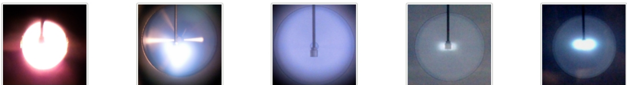
Figure 1. Reproducible plasma configurations. Left to right: He filling pressure decreases from (\sim 8 \rightarrow 2) \times 10^{-3} Torr, @RF 0.12 kW.
