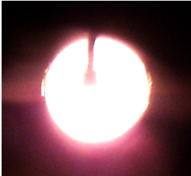
Figure 16. Plasma on port for  $p=9\times 10^{-3} Torr$  ,  $P=0.15kW$  .
