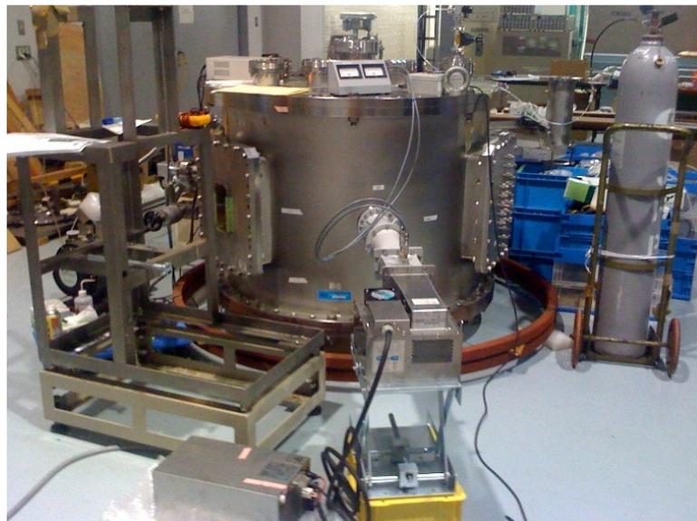
Figure 3. RF system and gas injection side of the vacuum chamber. On the bottom side the RF system can be seen along with its waveguide.
