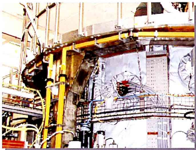
Figure 5.9: Photograph of the error field correction coil on MAST
