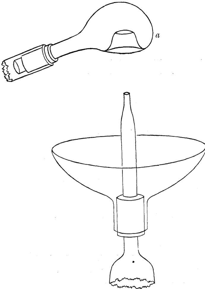
The liquid is filled into the pipette from below as usual; any excess of liquid is projected by its own force into the bulb above,
