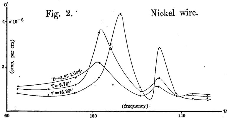
As will be seen from the figures, the maximum amplitude of vibration and the frequency corresponding to the maximum increase with weight. By altering the length of the ferromagnetic wire, the positions of the maxima and minima are but slightly affected.
