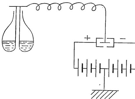
*Experiment I.*—The friction of sand particles with leaves, twigs, wood, etc. These objects were placed one by one upon the Mascart's insulator, and from a metallic funnel suspended by silk thread, a stream of fine sand was poured down against them, so as to electrify them by friction. In each case, the electrometer showed a positive electrification. These objects were then disconnected from the wire, and held by a separate stand over the insulator. A stream of sand
