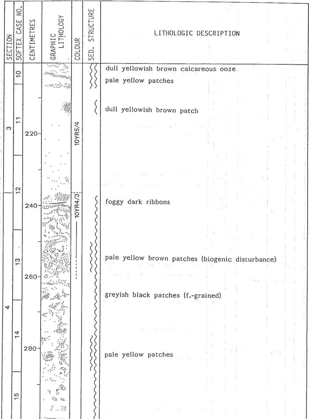
Fig. 14.2c Visual description of piston core KH92-1 2PC (200 - 300 cm).
