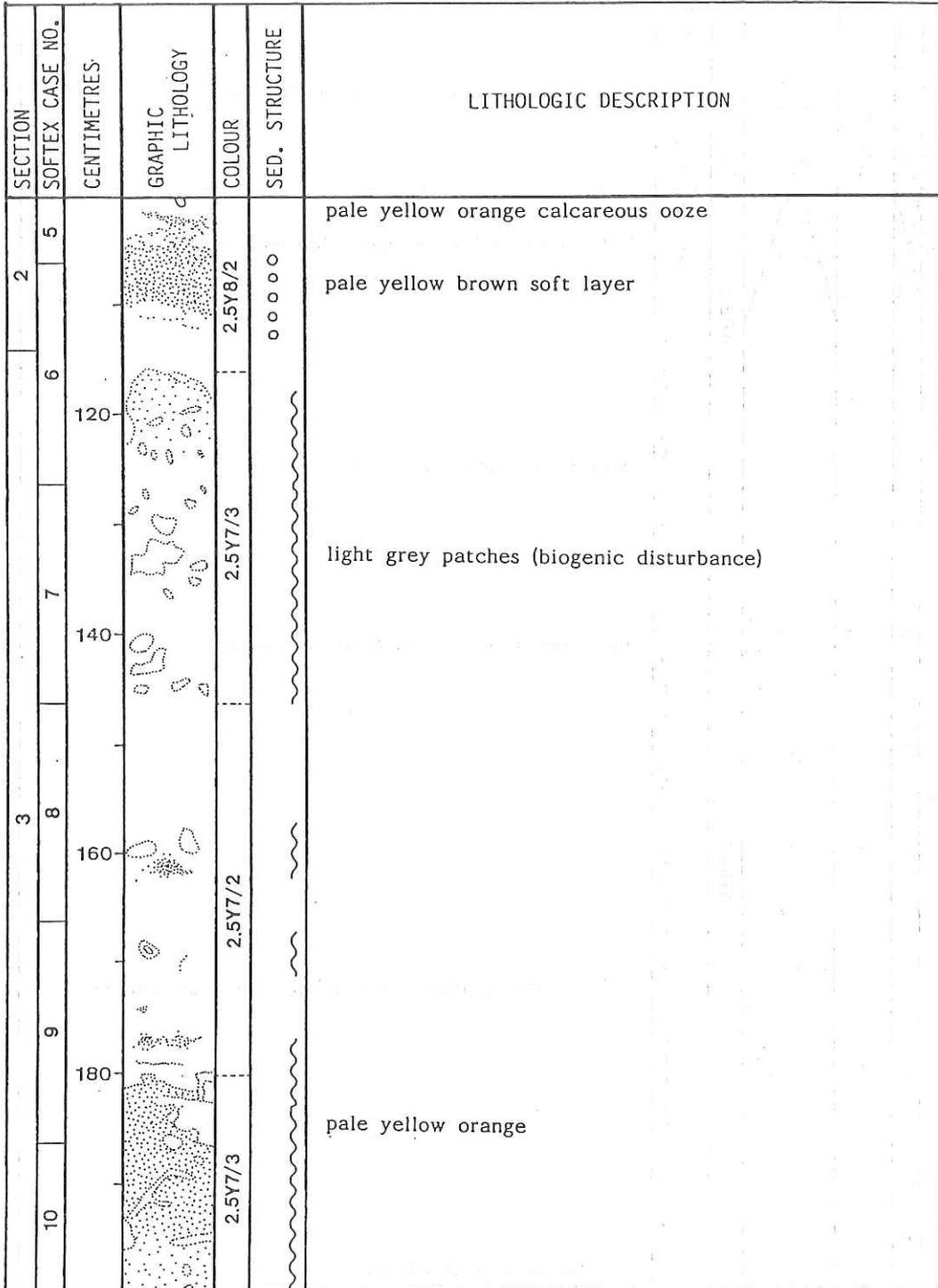
Fig. 14.3b Visual description of piston core KH92-1 3aPC (100 - 200 cm).
