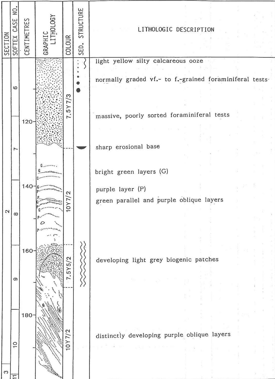
Fig. 14.7b Visual description of piston core KH92-1 2PC (100 - 200 cm).
