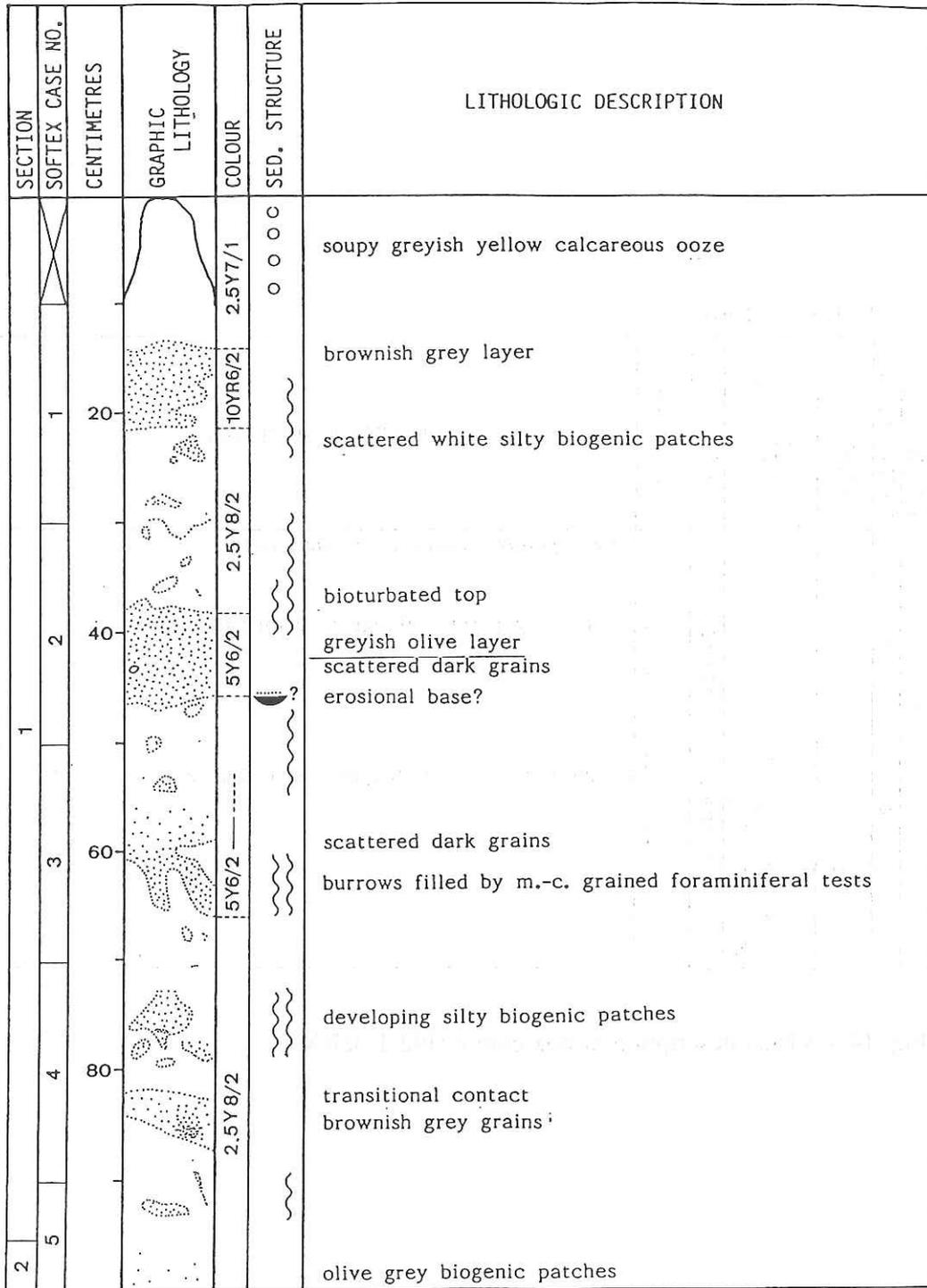
Fig. 14.5a Visual description of piston core KH92-1 5aPC (0 -100 cm).
