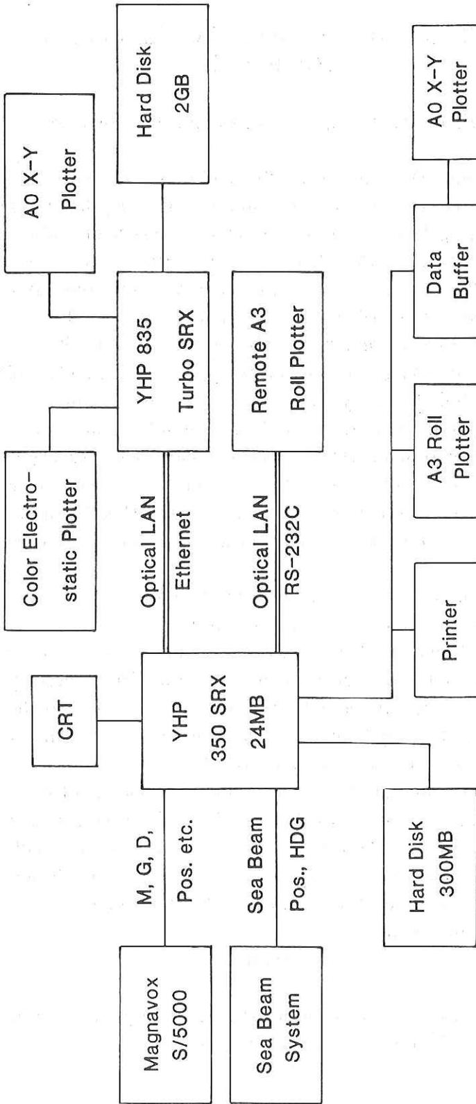
Fig. 6.1.2 Real-time mapping system on board the Hakuho-maru.
