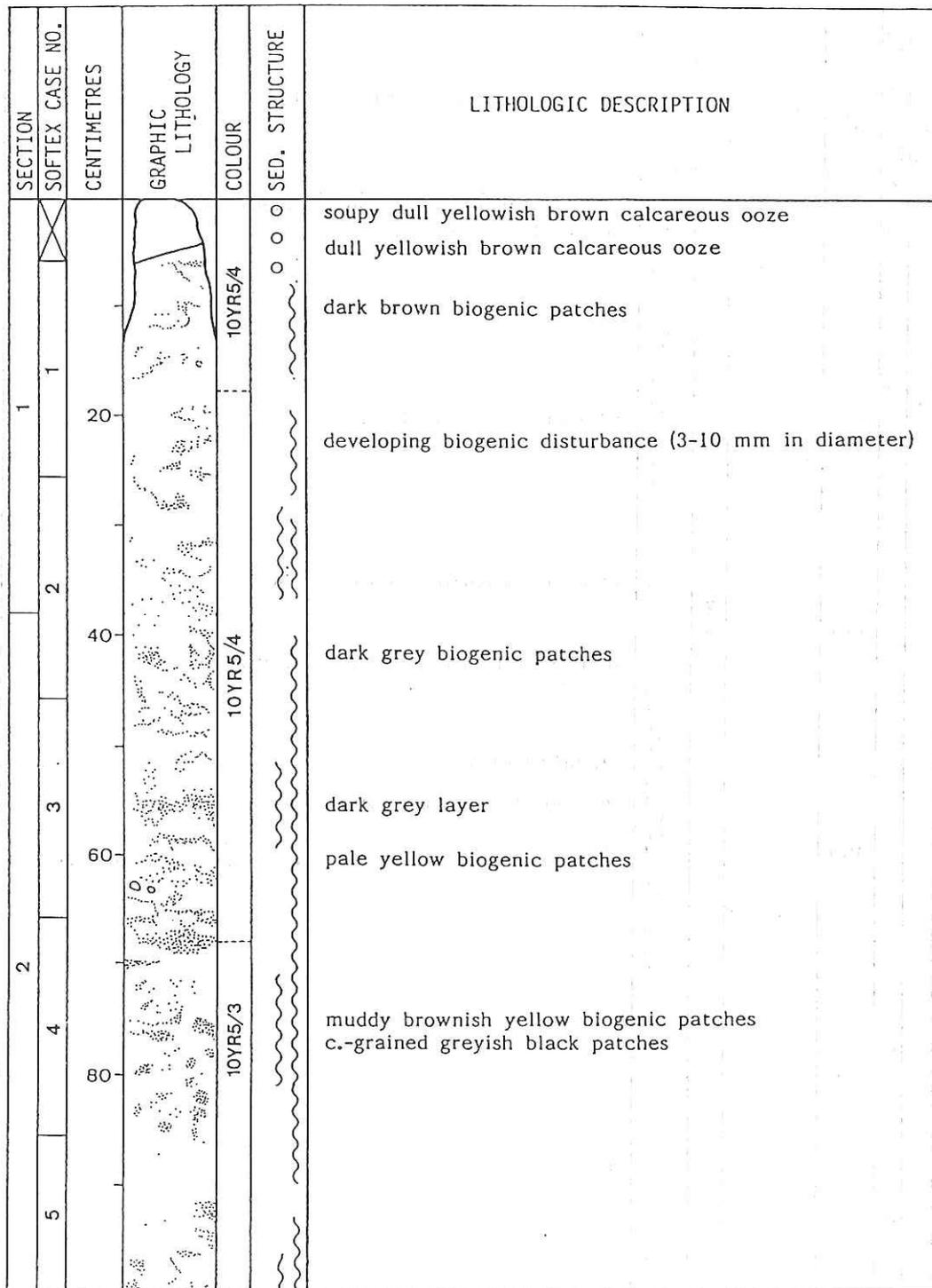
Fig. 14.2a Visual description of piston core KH92-1 2PC (0 - 100 cm).
