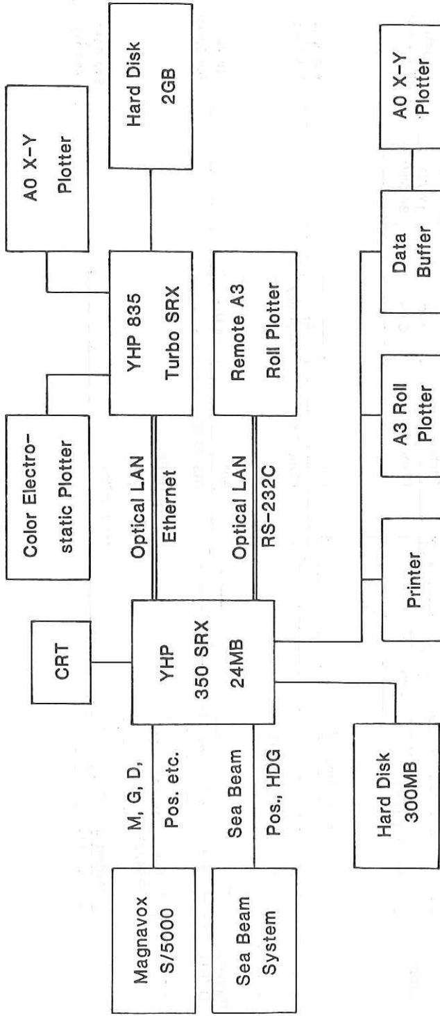
Fig. 4.2.3 Block diagram of the Real-time Mapping System on board the Hakuho-maru.
