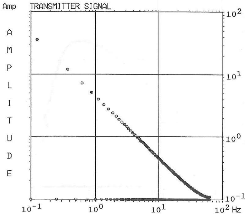
Fig. 4.6.4.3. The amplitude spectra of the transmitter signal. From the 40 Amperes commutated square wave form the FFT's result shows odd harmonics only.
