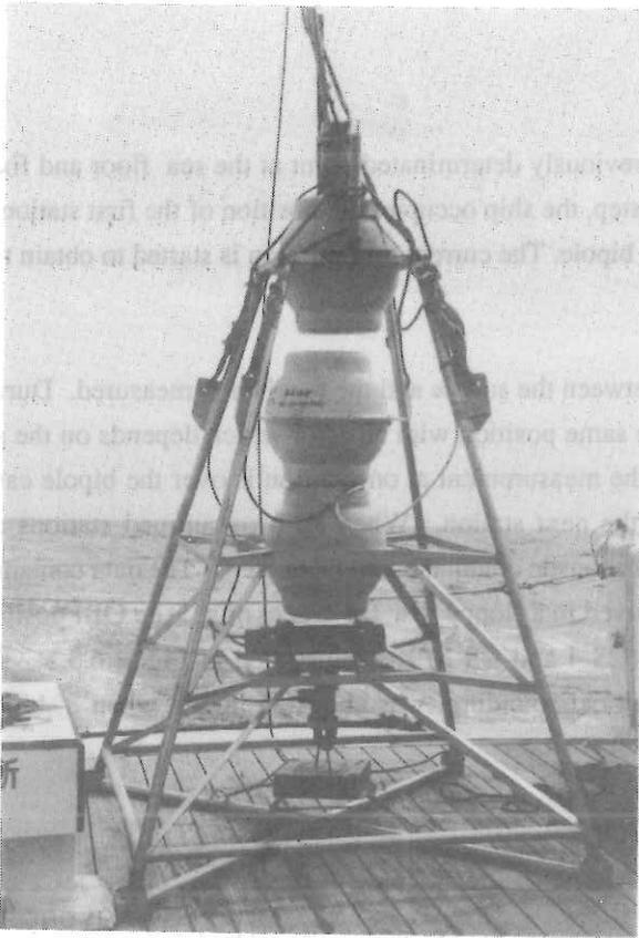
Fig. 4.6.3.4 The receiver (OBI). Three Benthos spheres mounted on the aluminum frame assure the buoyancy. The upper sphere contains the sensor, the lower the electronics. At the top of the frame are attached a flasher, a radio beacon and a transducer and at the base a plumb anchor, a release system and a transponder.
