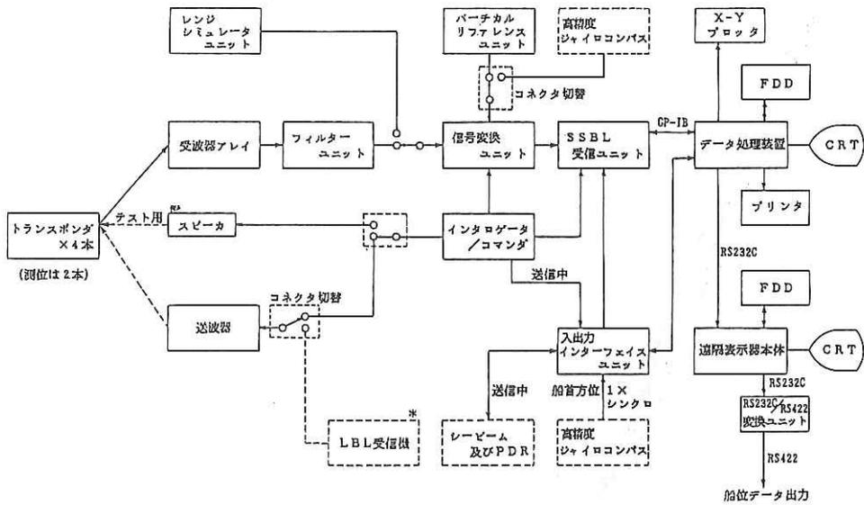
Fig. 4.10.1 Block diagram of the SSBL transponder system.
