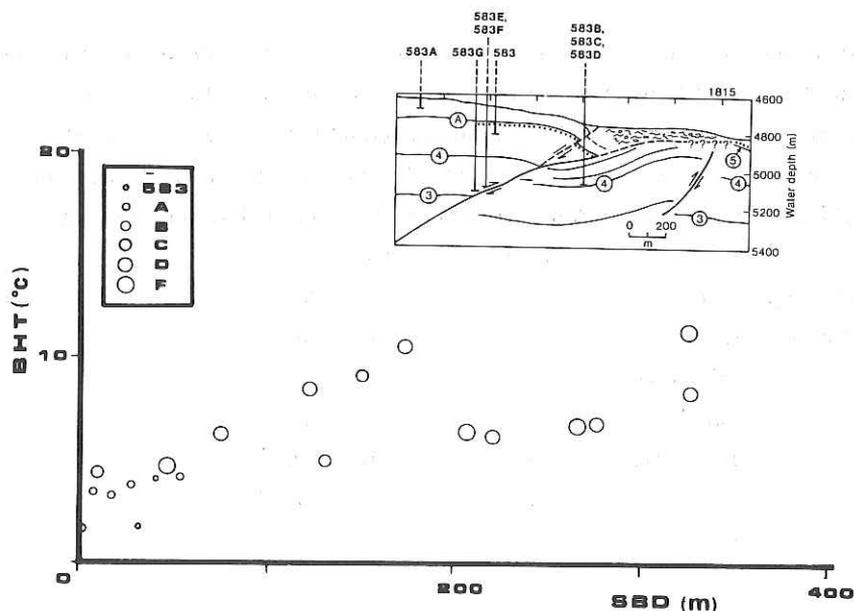
Fig. 4.11.A-3: Bottomhole temperatures (BHT) versus subbottom depths (SBD) measured in Leg 87, DSDP (Kagami and Karig et al., 1986). Top insert shows relative positions and depths of each holes measured. Hole assignments are given as legend in a frame on left side.
