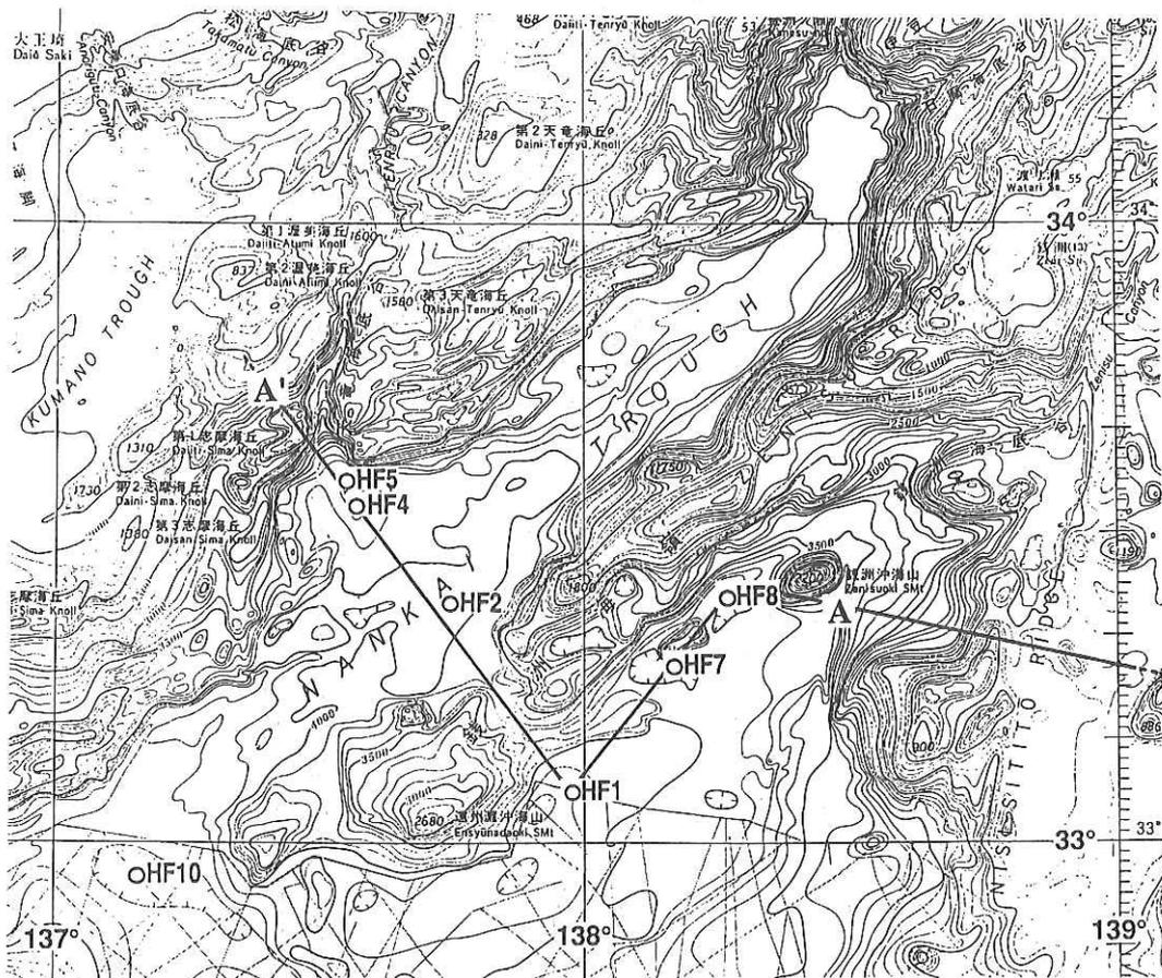
Fig.4.8.1 Position of heat flow station plotted on a bathymetry map. Line A-A' indicates track line, and 3.5kHz subbottom profile along this line is shown in Fig. 4.8.2.
