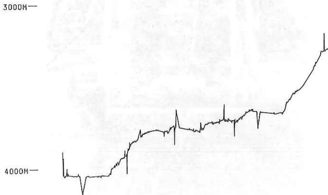
Fig. 4.10.4 Vertical section of positions (depth) of the sub-navigation transponder.
