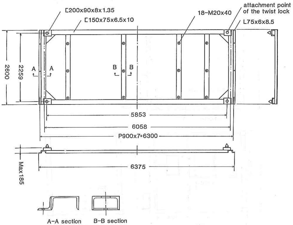
Fig. 5.2.3.4 Plan of attachment base for the container to operate TV camera system.
