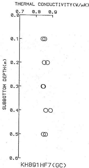
Fig.4.8.4 A thermal conductivity versus depth profile at HF-7.
