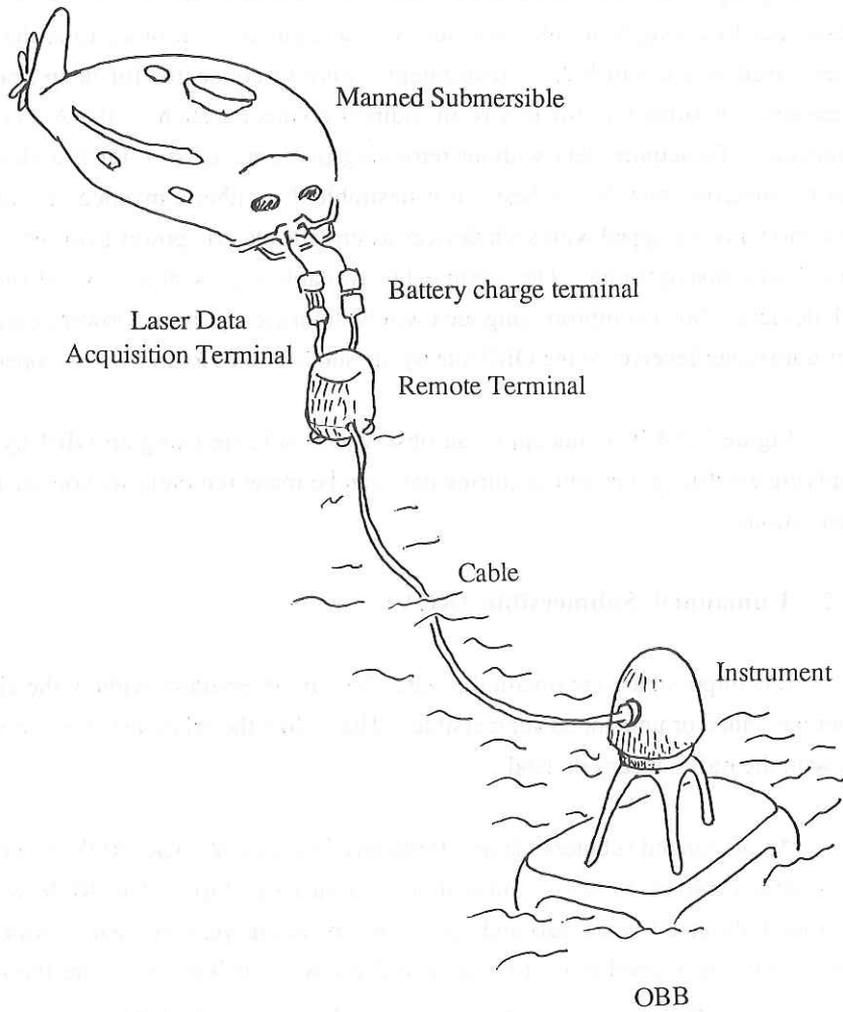
Fig. 3.2.4 An idea of OBB which is equipped with a battery charger and data transmission device.
