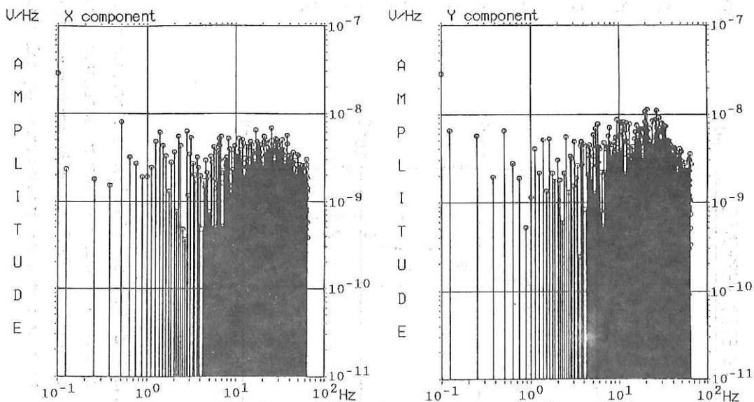
Fig. 4.6.4.6 Amplitude spectra of recorded noise of the OBI at the sea floor. Represents internal electronic "white" noise.
