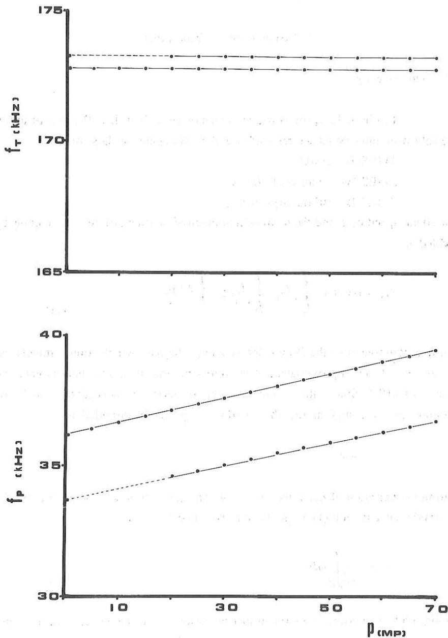
Fig. 4.11.A-5(1) and (2): Frequency change with hydrostatic pressure of high resolution quartz temperature sensor (1). Same for pressure sensor (2). Measurements were run at room temperature (15-16 deg. C). Frequency is in kHz, and pressure is in MPa.
