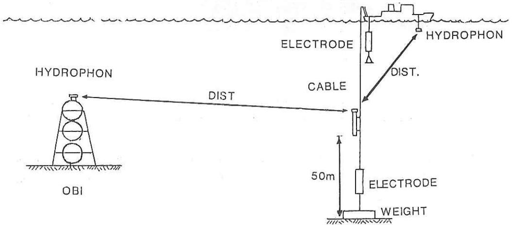
Fig. 4.6.3.3 A view of the MOSES experiment. The transmitter is a vertical insulated current - carrying cable extending from the sea surface to the sea floor. A large electrode and BRS's transponder are attached at the sea floor end of the cable. OBI is deployed at a point of distance  $r$ , which has another transponder. The distance  $r$  is measured and registered periodically on the ship by means of acoustic signals.
