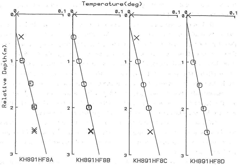
Fig.4.8.3 Temperature versus depth profiles. A straight line is the best fit line for data except for cross-mark (x) ones, which mean that they did not penetrate, or the record was unstable. Depth values are corrected for the instrument tilt.
