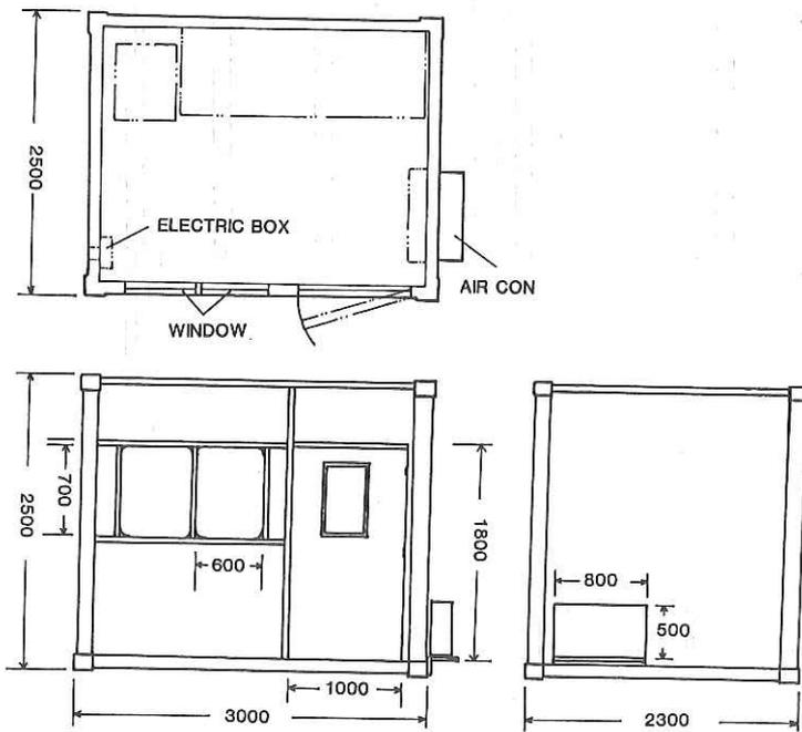
Fig. 5.2.3.2 Plan of container for operating side scan sonar system.
