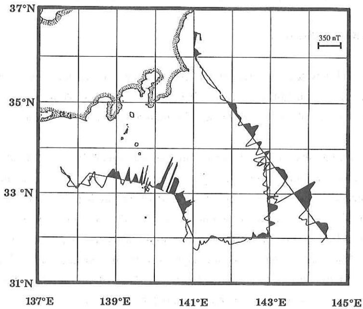
Fig. 4.3.3 The magnetic anomaly profiles along tracks (reference field IGRF 1985). Portions of positive anomalies on the profiles are painted black.
