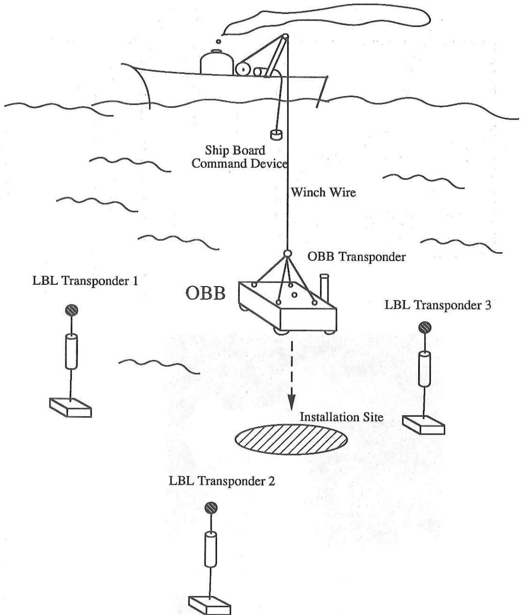
Fig. 3.2.1 A schematic illustration of Long Base Line Positioning Method and Subnavigation Method.
