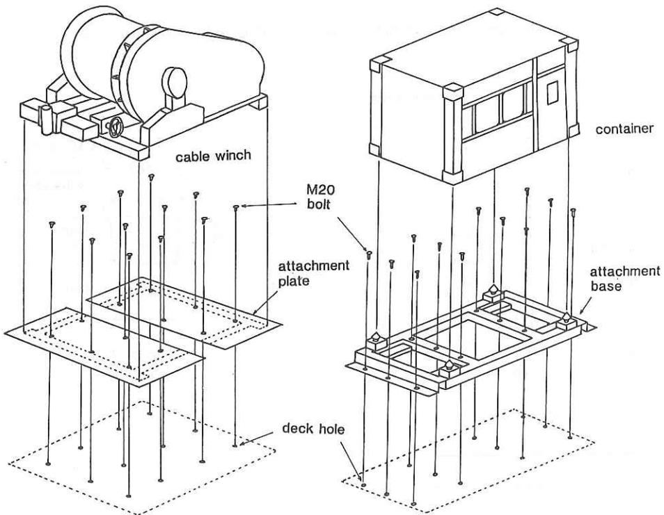
Fig. 5.2.3.8 Block-diagram of setting the cable winch (left) and the container (right).
