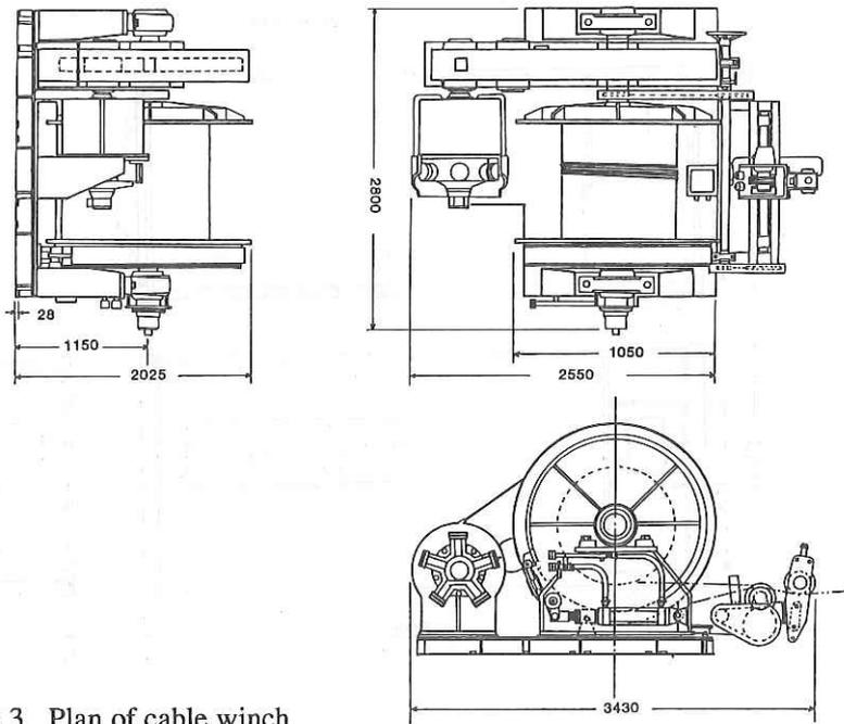
Fig. 5.2.3.3 Plan of cable winch.
