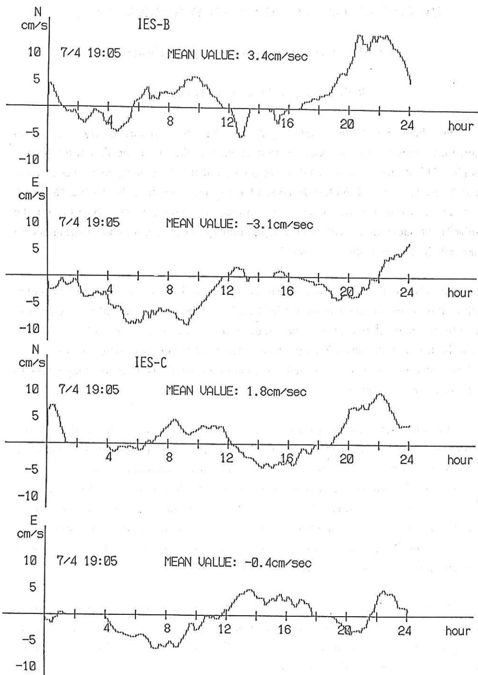
Fig.4.12.4 Currents measured by Aanderaa current meters at the depth of 1700 m.
