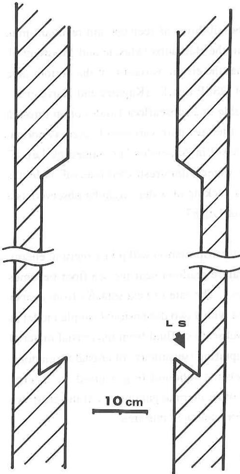
Fig. 4.11.3: Cross-section of a landing sub (LS with a thick arrow) carved on a wall of casing in a shape of a niche. Approximate scale is given in bottom center in unit of cm.
