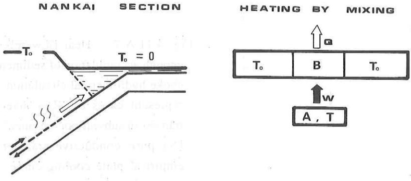
Fig. 4.11.A-4: Schematic cross-section of Nankai Trough (left). Subducting plate squeezes some fluids upward while rupture occurs deep in the subseafloor faults. Seafloor temperature is kept approximately constant and equal to 0 degree C. Two dimensional model is assumed. Mixing of warm fluid (right) with top sediment cover produces heat flow ( $Q$ ) higher than that of surrounding area. Parameters used for this model are:
