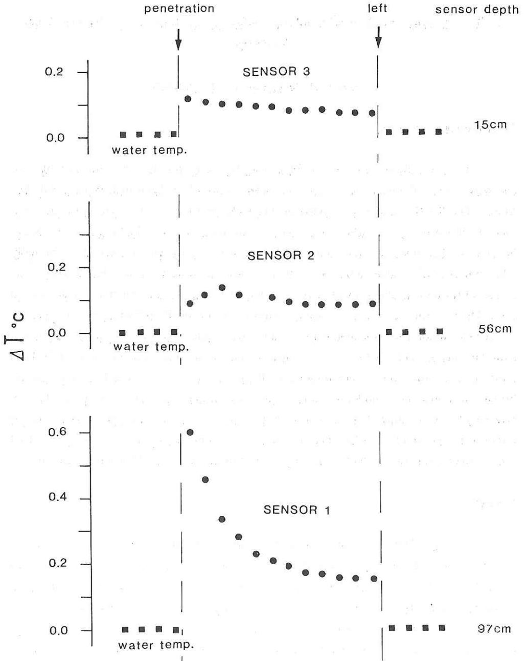
Fig. 4.9.1 Temperature variation of each heat sensor before and after penetration into sediment. The ordinate shows variation of temperatures ( $\Delta T^{\circ}\text{C}$ ) of each sensor, and abscissa shows measuring time (full scale approximately 15 minutes); interval of each data telemetry is about 30 to 45 seconds.
