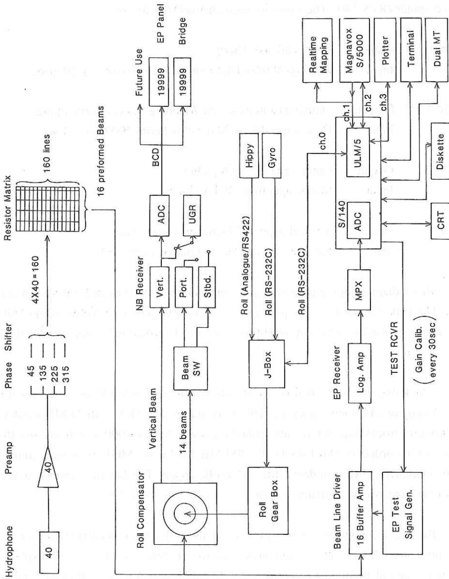
Fig. 4.2.1 Block diagram of the Sea Beam signal processing.
