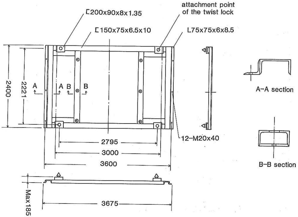
Fig. 5.2.3.5 Plan of attachment base for the container to operate side scan sonar system.
