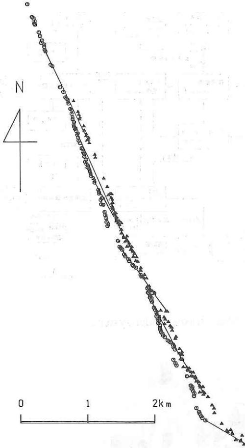
Fig. 4.10.3 Tracks of the ship and subnavigation transponder. circle: ship position, triangle: subnavigation transponder position. Tie line shows the simultaneous positions of ship and deep tow.
