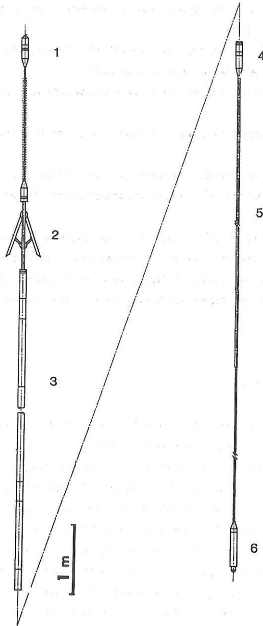
Fig. 4.11.2: Schematic illustration of ONDO. From top left (1) through bottom right (6) are; (1) Acoustic element, (2) Landing pad, (3) Pressure housing with power supply, data processor and data logger, (4) Connector of thermistor cable with data processor, (5) Thermistor cable (800 meters) with 19 sets of ceramic thermistor, and (6) Pressure gauge and a dead weight below it. Approximate scale of dimension is given in bottom left in unit of meters.
