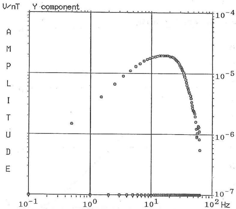
Fig. 4.6.4.2 The Amplitude Spectra of the OBI's Response Function for X and Y components.
