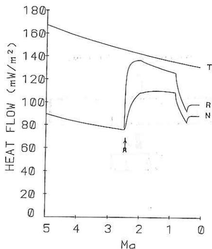
Fig. 4.11.A-2: Heat flow rebound after enough accumulation of sediment cover to choke hydrothermal circulation. R and N represent cases of (R) convective heat transfer in subseafloor basement layer, and (N) pure conductive transfer. T is empirical plate cooling curve. Further details are referred to in Nagihara et al. (1989).
