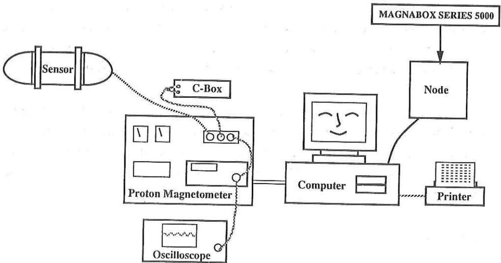
Fig. 4.3.1 Block diagram of the measurement of the geomagnetic total force.
