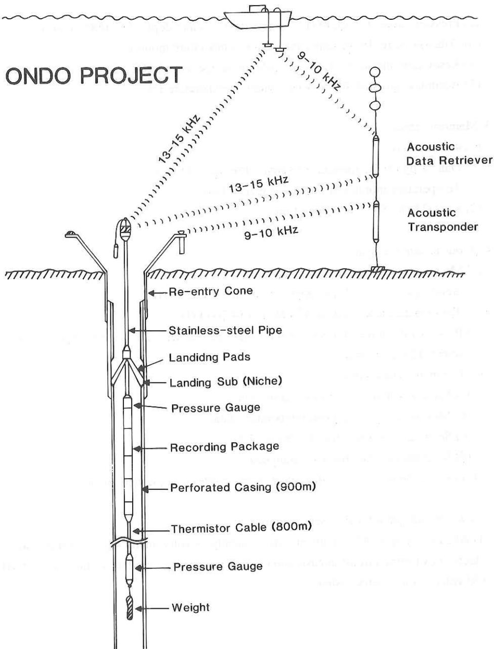
Fig.4.11.4: The temperature monitoring system after the deployment and data retrieval with surface vessel. A transponder is used also for range measurement to the re-entry cone. Acoustic data retriever (right) sitting on the sea floor receives data on carrier frequency of 13-15kHz transmitted from the downhole system (ONDO) according to "Send Data" command (9-10kHz) from the surface ship. It surfaces after retrieval of the ONDO data by use of a releaser of the acoustic transponder.
