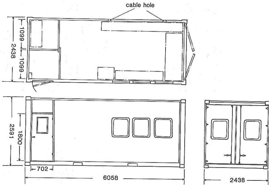
Fig. 5.2.3.1 Plan of container for operating TV camera system.
