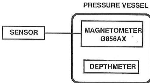
Fig. 4.4.1 Block diagram of the ORI-DTP I (Ocean Research Institute Deep Towed Proton-magnetometer) system.
