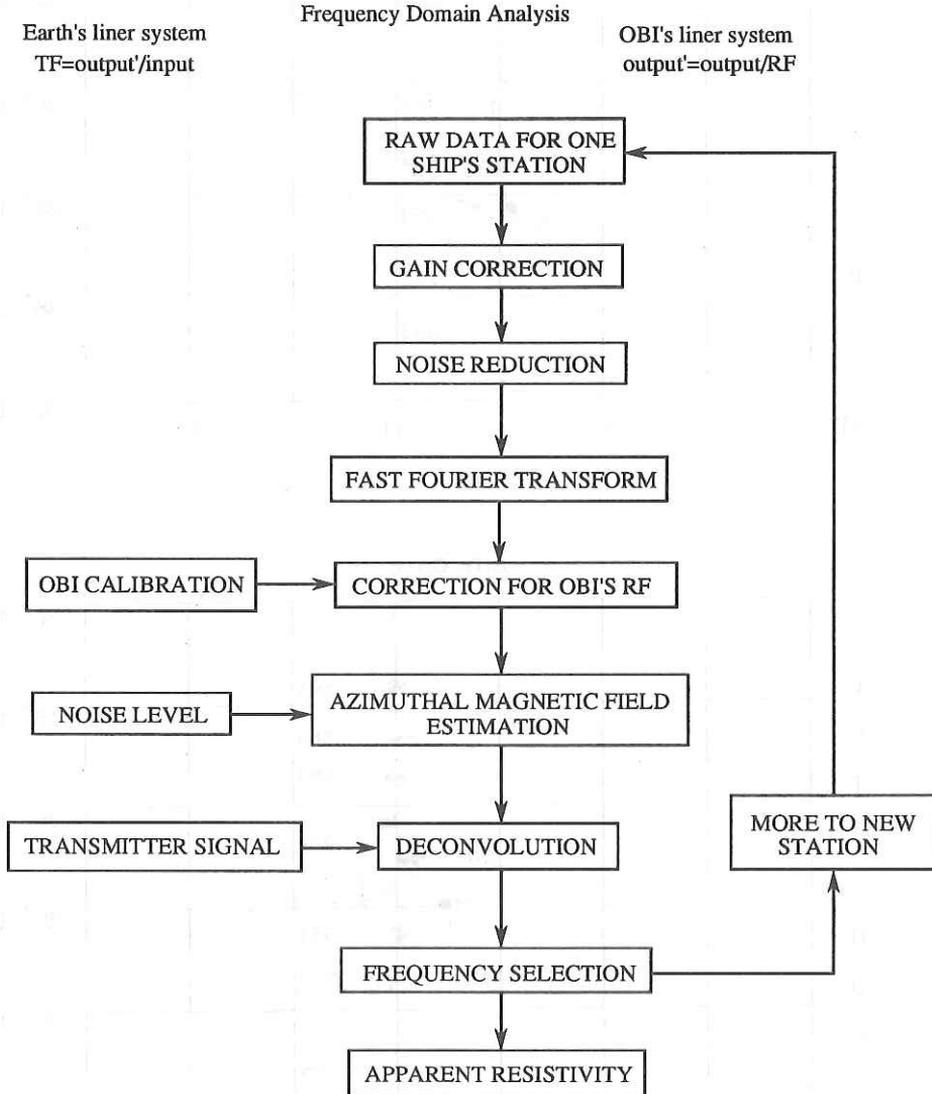
Fig. 4.6.4.1 The schematic diagram to obtain the azimuthal magnetic transfer function of the earth from the two linear systems concatenated. The input at OBI is equal to the earth's output. Also the flow chart of data processing from the output raw data to the apparent resistivity versus source receiver distance for the selected frequency is shown.
