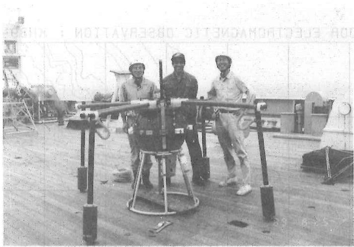
Fig 4.7.2 A photograph of OBEM just before launch on board.
