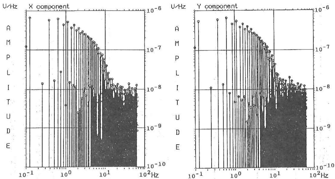
Fig. 4.6.4.5 Amplitude spectra of recorded data for X and Y components. The signal is contained in the odd harmonics.
