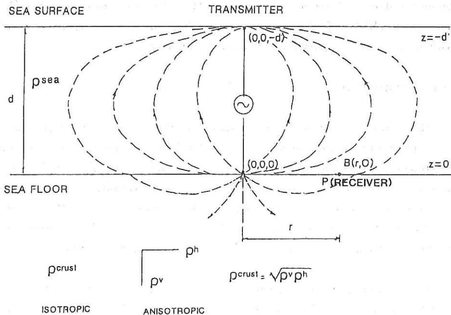
Fig. 4.6.2.1 General scheme of the MOSES method. The electric current flows from the sea surface to sea floor through a cable and returns through sea water. Some current penetrates in the crust and returns to the sea surface. This currents have a vertically symmetric axis and are proportional to the resistivity contrast between the sea water and the crust. The azimuthal magnetic field measured at the sea floor is proportional to the amount of current enclosing the field point P.
