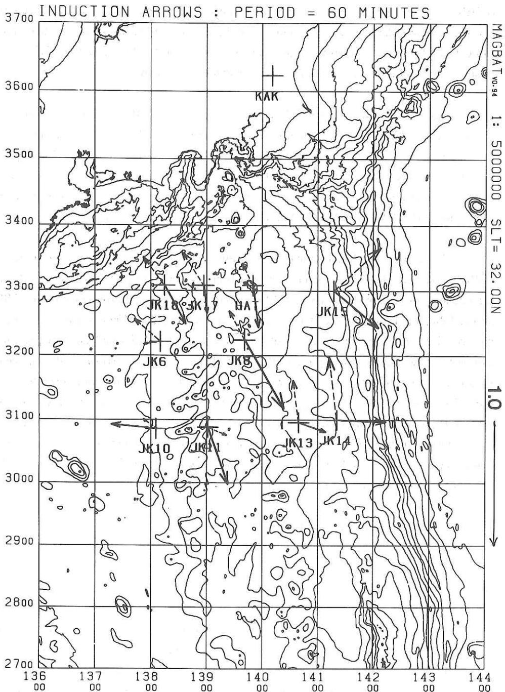
Fig 4.7.1 Mapping of the induction vectors around the Izu Bonin ridge for the period of 60 minutes. The induction vectors were calculated from the data obtained during the previous three cruises; KT86-12, KH87-3 and KT88-10. Solid arrows indicate the real parts of the calculated transfer functions, while dashed arrows denote imaginary ones.
