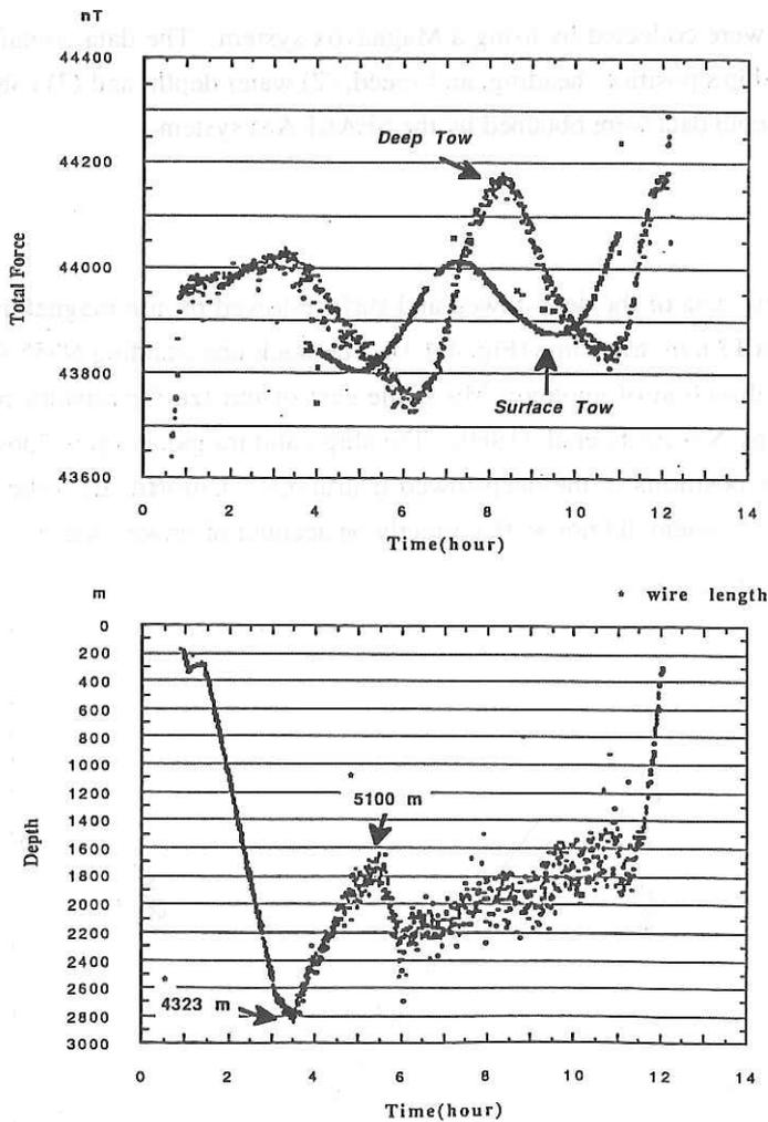
Fig. 4.4.4 Profiles of magnetic total field intensities obtained by the deep-towed and surface-towed proton magnetometers (upper). Transponder depth determined by an acoustic transponder navigation system (lower).
