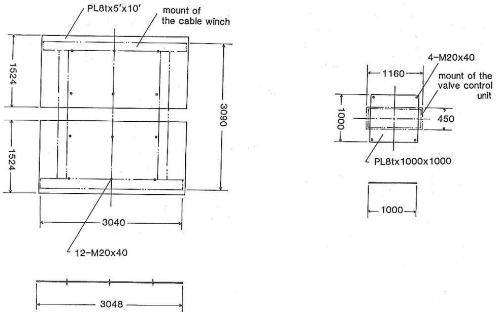
Fig. 5.2.3.6 Plan of attachment plate for cable winch (left) and control valve unit (right).
