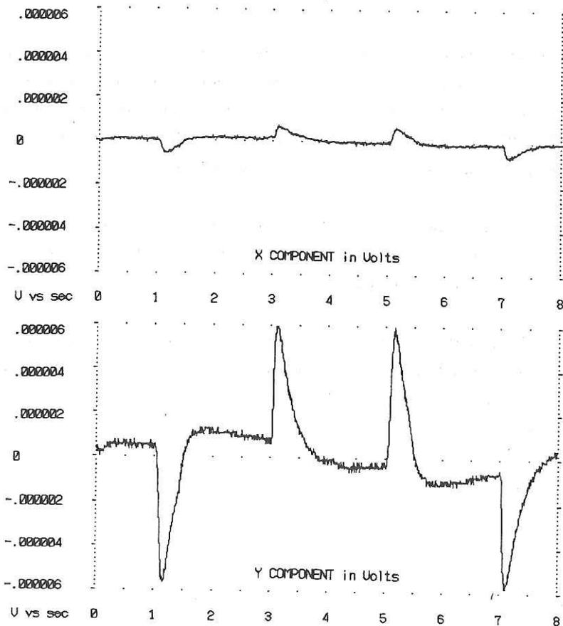
Fig. 4.6.4.4 The stacked time series recorded at OBI (site CS-4) for X and Y components at the station SN1 (370 m between source - receiver).
