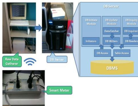
Fig.2. Power monitoring system. Smart metering device send power measures to raw data gatherer via wireless network, DB server periodically fetch raw data and update it into database. The data is stored for later inquiries.
