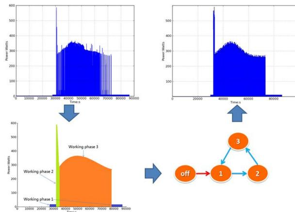
Fig.6. Making of profiles for air conditioner class appliance: 1.Capturing of practical power data using PMS (upper left), 2.Deciding abstracted working phases (lower left), 3.Making transition chart (lower right), 4.Comparing the simulation data.
