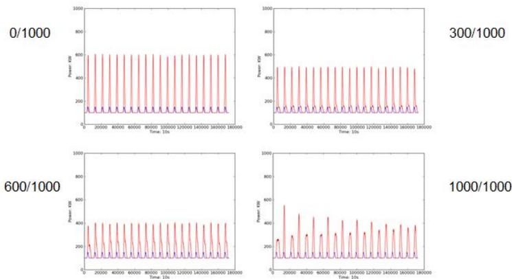
Fig.13. Power curves with different number of schedulable tasks, the number beside is the portion of schedulable tasks in non-emergent tasks
