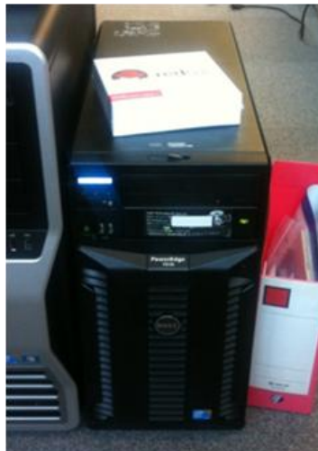
Fig.2.6. Database server, Dell PowerEdge T310
