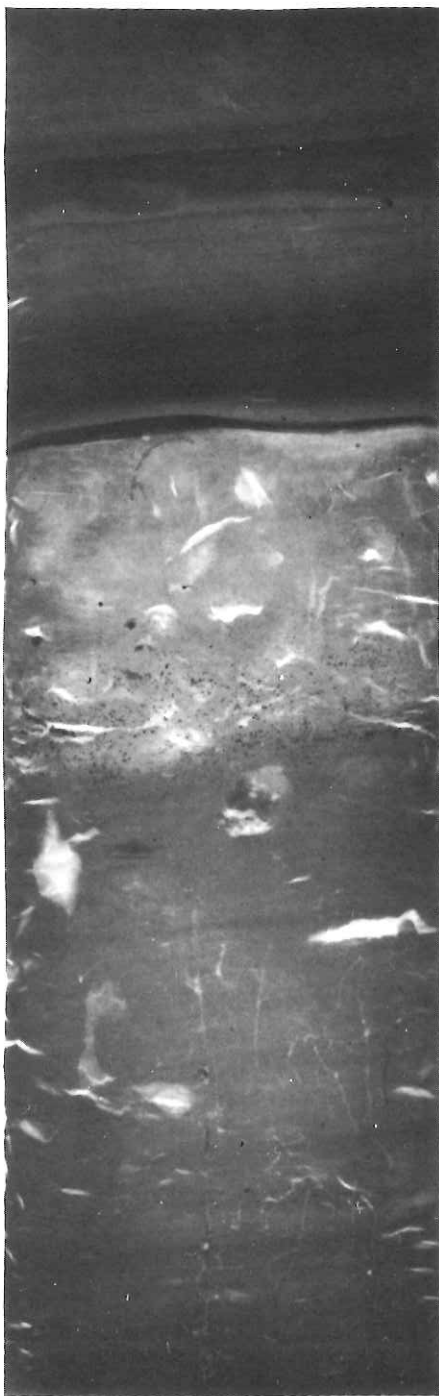
Fig. 1 a X-ray radiograph of laminated sediment of Nankai Trough axis floor. KH-86-5 P6 132-152cm. The upper 6cm is turbiditic layers, but the other part is hemipelagic laminated mud. Many crevices by generated gasses are distinct.
