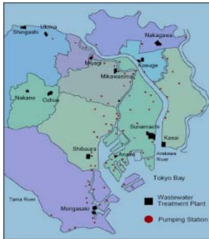
Fig. 1.2 Tokyo waste water treatment plant and pumping stations
