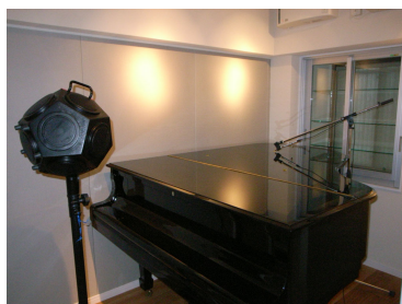
Fig. 5.2 Speaker and microphone for measurement.
