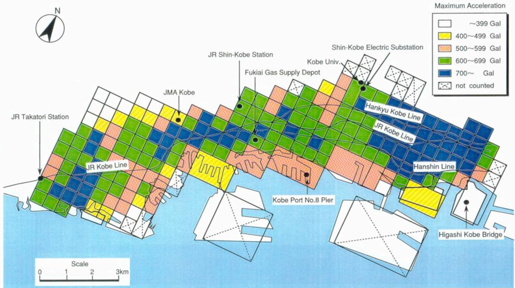
Fig.6 Distribution of maximum acceleration for macro-analysis based on Sato's results 15)
