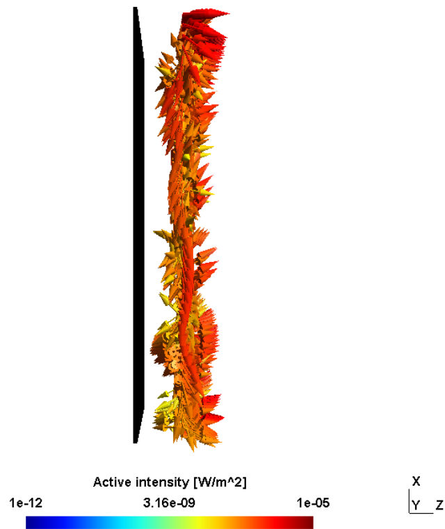
Fig. B.11 Distributions of sound intensity at 1224 Hz, (l_1, l_2) = (0.1, 0.25) , h_p = 10 mm, d_m = 0.1 m, incident angle: (\theta, \varphi) = (75^\circ, 0^\circ) .
