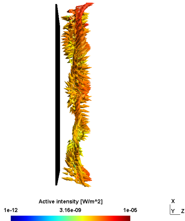
Fig. B.2 Distributions of sound intensity at 1224 Hz, (l_1, l_2) = (0.1, 0.25) , h_p = 10 mm, d_m = 0.1 m, incident angle: (\theta, \varphi) = (15^\circ, 0^\circ) .
