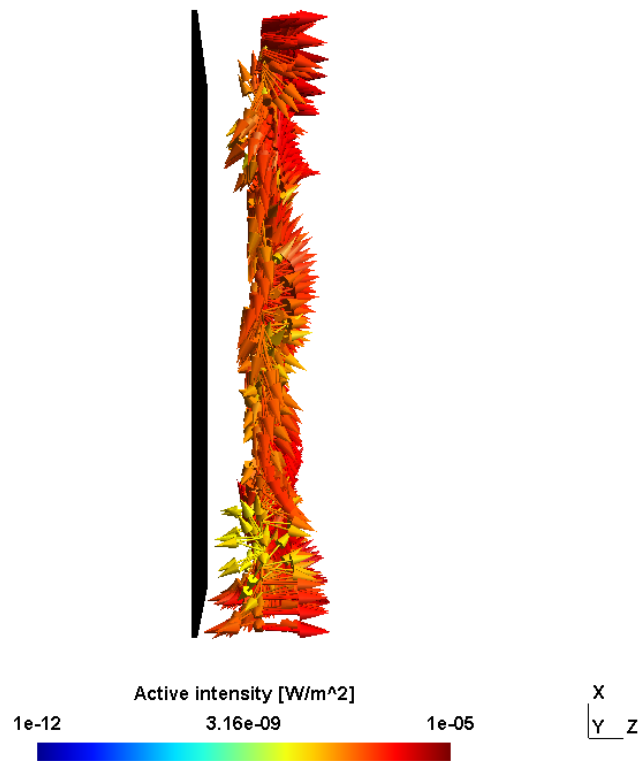
Fig. B.8 Distributions of sound intensity at 1224 Hz, (l_1, l_2) = (0.1, 0.25) , h_p = 10 mm, d_m = 0.1 m, incident angle: (\theta, \varphi) = (45^\circ, 0^\circ) .
