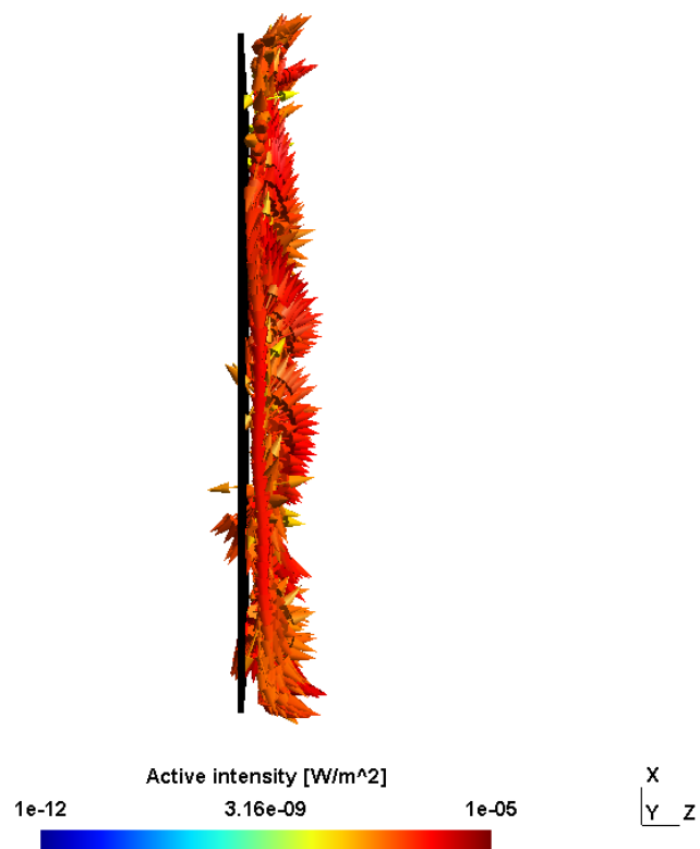
Fig. 4.31 Distributions of sound intensity at 1224 Hz, (l_1, l_2) = (0.1, 0.25) , h_p = 10 mm, d_m = 0.025 m, incident angle: (\theta, \varphi) = (60^\circ, 0^\circ) .
