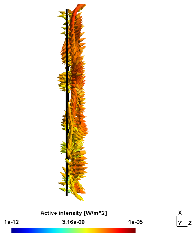
Fig. B.1 Distributions of sound intensity at 1224 Hz, (l_1, l_2) = (0.1, 0.25) , h_p = 10 mm, d_m = 0.025 m, incident angle: (\theta, \varphi) = (15^\circ, 0^\circ) .
