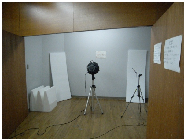
Fig. 3-3 Position of a source and receiving point in the warehouse.
