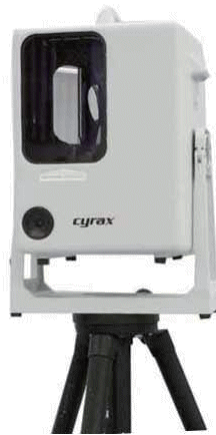
Figure 5.14: The range sensor Cyrax 2500 used to acquire the shape information.
