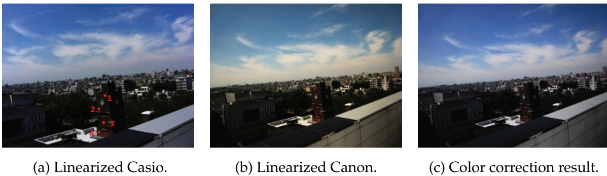
Figure 3.12: Color correction between different cameras: (a) is the target image captured by Casio, (b) is the source image captured by Canon, (c) shows the color correction result from Canon (b) to Casio (a).
