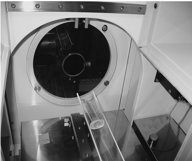
**Fig. 2.** 3D micro X-ray CT sample stage.
