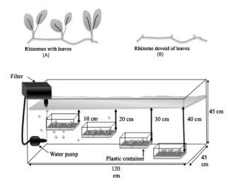
**Fig. 1.** The planting materials, rhizome axes with leaves (A) or rhizome axes devoid of leaves (B) are planted in a substrate in plastic containers, immersed at different depths in a culture system (C) containing artificial seawater.
