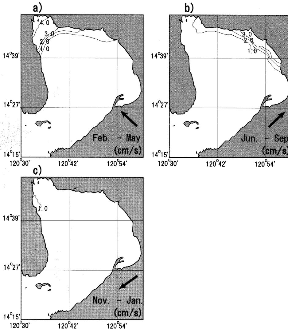
**Fig. 5.** Horizontal distribution of water velocity amplitude above the bottom due to wind waves in Manila Bay from February to May (a), from June to September (b) and from November to January (c). Contour interval is  $1.0 \text{ cm} \cdot \text{s}^{-1}$ . Thick arrow shows wind direction at Manila.
