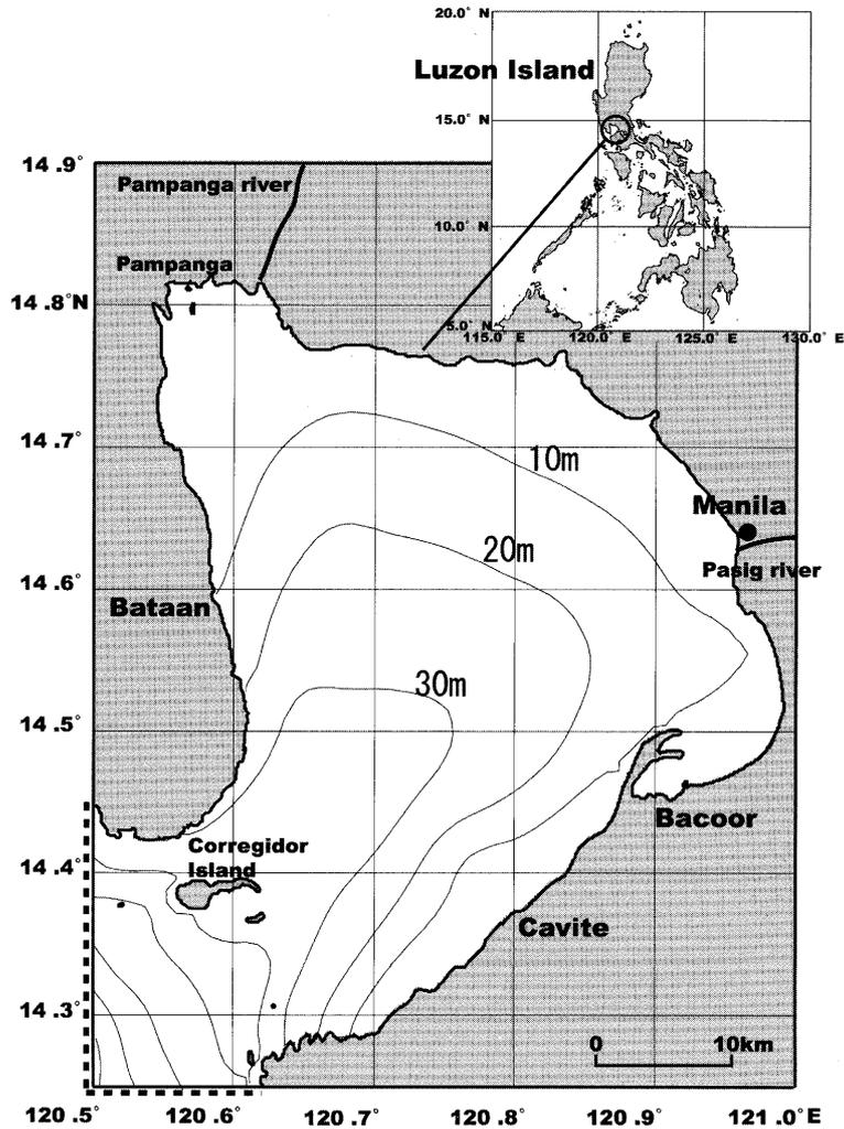
**Fig. 1.** Model area with bathymetry. Closed circle shows the tide gauge station. Broken line shows the open boundary of the numerical model, and thick lines show rivers flowing into Manila Bay.
