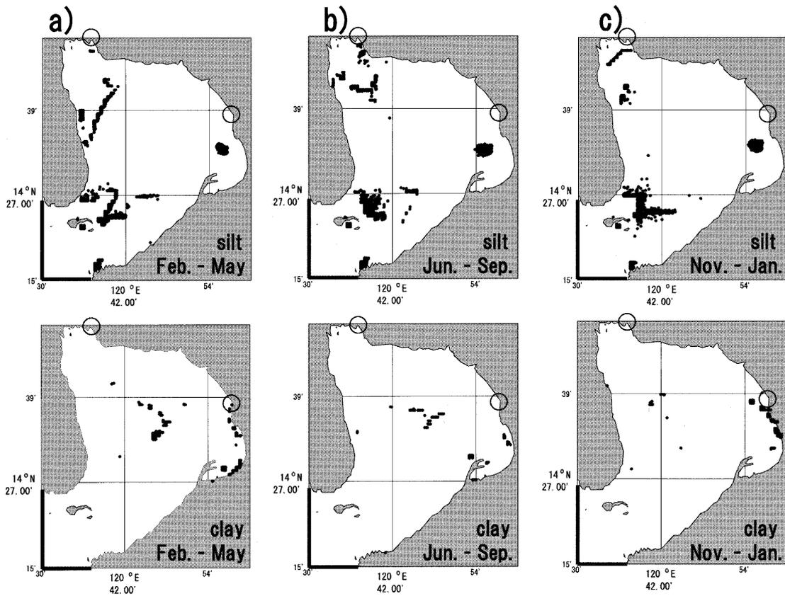
**Fig. 6.** Calculated horizontal distributions of deposited silt and clay from February to May (a), from June to September (b) and from November to January (c). Open circles and thick line denote the injection points. Black circles represent accumulated particles.
