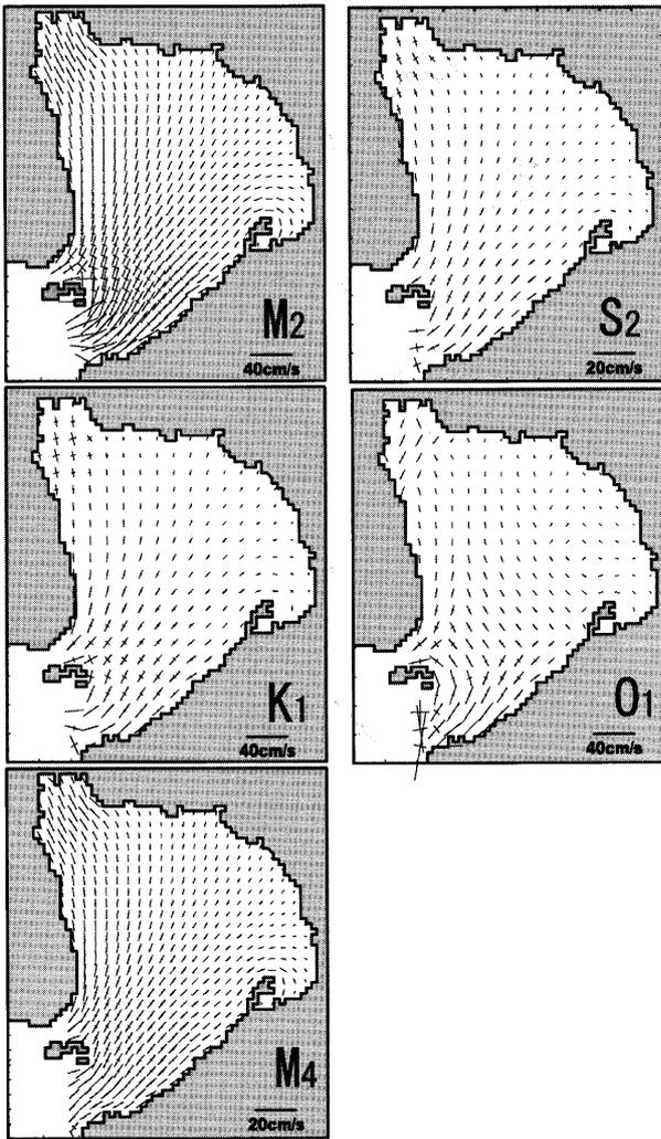
Fig. 2. Calculated long and short axes of  $M_2$ ,  $S_2$ ,  $K_1$ ,  $O_1$  and  $M_4$  tidal current ellipses (Fuji-ie et al. 2002).
