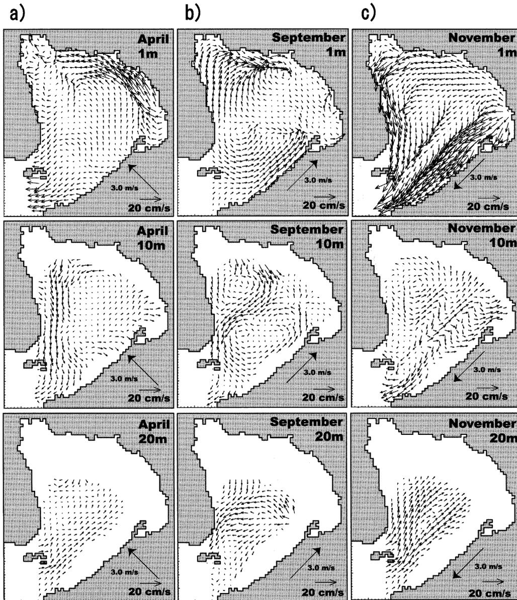
**Fig. 4.** Calculation results of residual currents from February to May (a), from June to September (b) and from November to January (c). Thick arrow represents wind direction (Fuji-ie et al. 2002).
