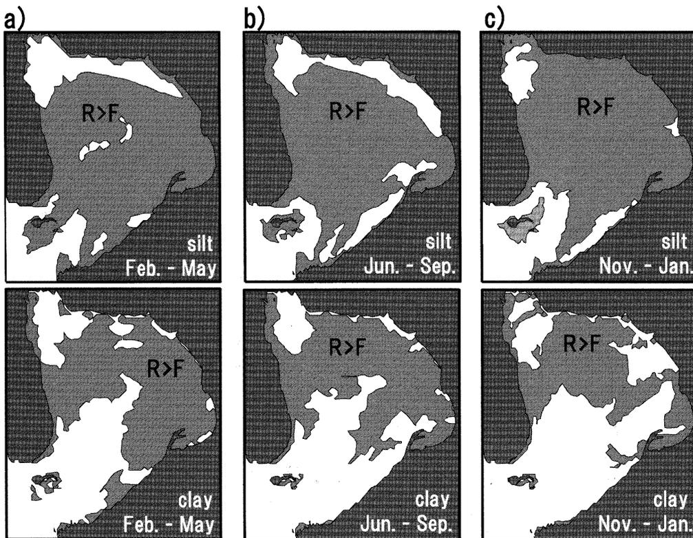
**Fig. 7.** Comparison of tractive and resistance forces from February to May (a), June to September (b) and November to January (c), respectively. Shadow region shows the area where the resistance force is larger than the tractive force and white area the opposite case.
