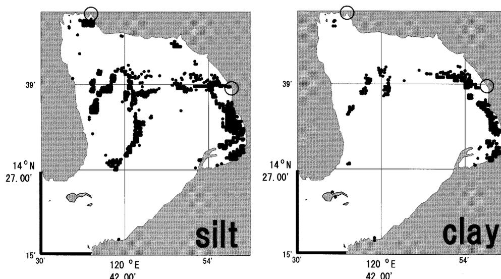
**Fig. 8.** Horizontal distributions of deposited silt and clay throughout the year in Manila Bay. Open circles and thick line denote the injection points. Black circles represent accumulated particles.
