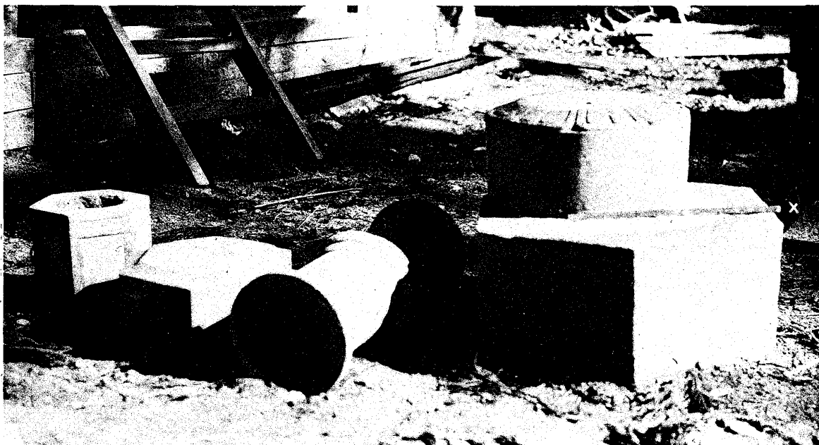
Fig. 4. A Stone-lantern overturned, at Jokoji (常光寺) Temple, Yashiro-mra. (X) .... A foot-scale indicating the amount of the displacement of the pedestal.
