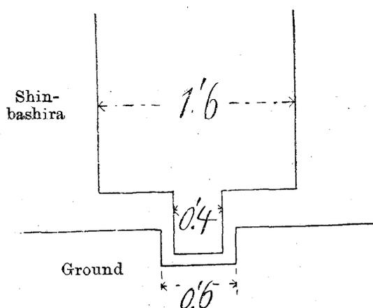
Fig. 13. Section of the lower end of the Central Post Pendulum of the Asaksa Gojunoto.
