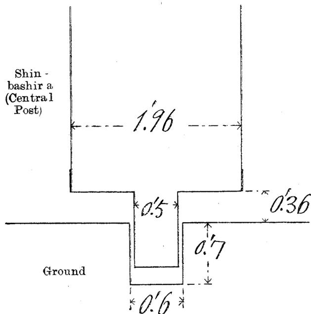
Fig. 12. Section showing the lower end of the Central Post Pendulum of the Nikko Gojunoto.
