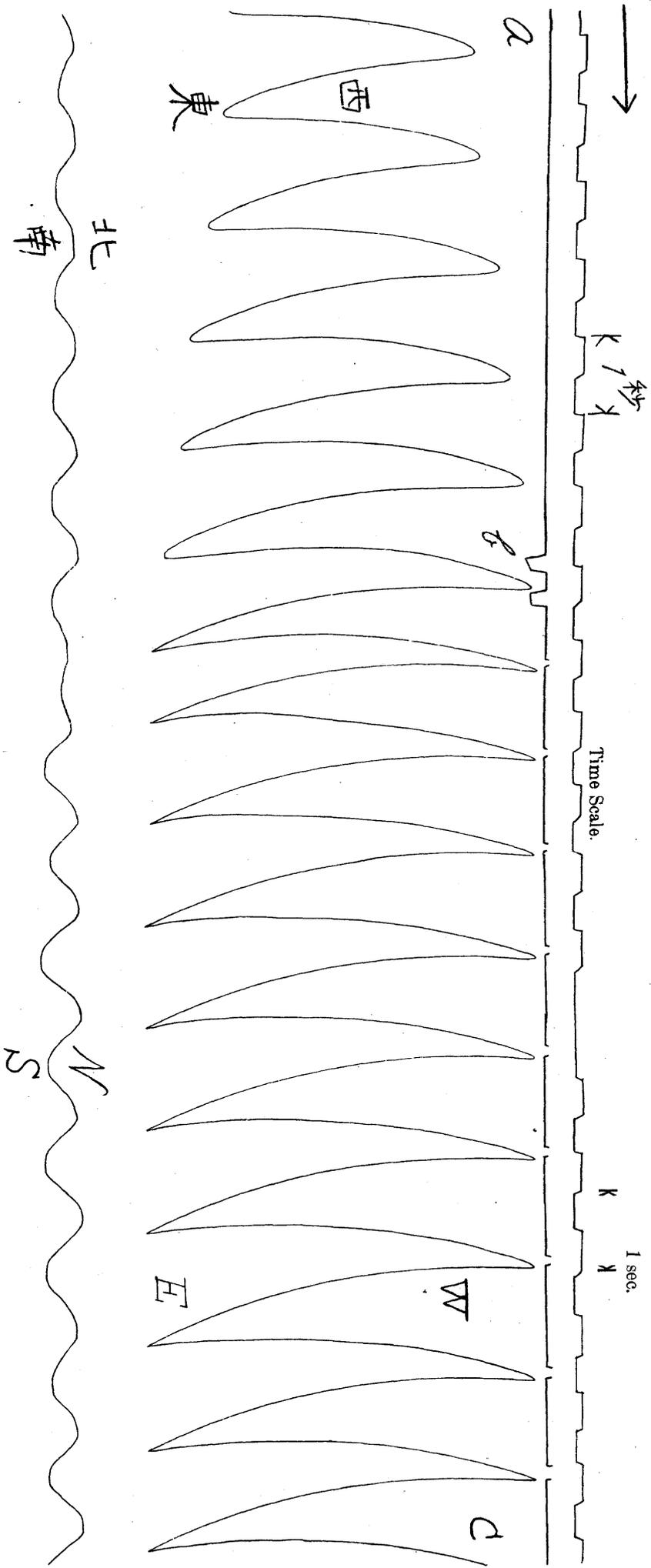
Fig. 23. Vibration of the Hommonji Gojunoto Caused by Wind.
