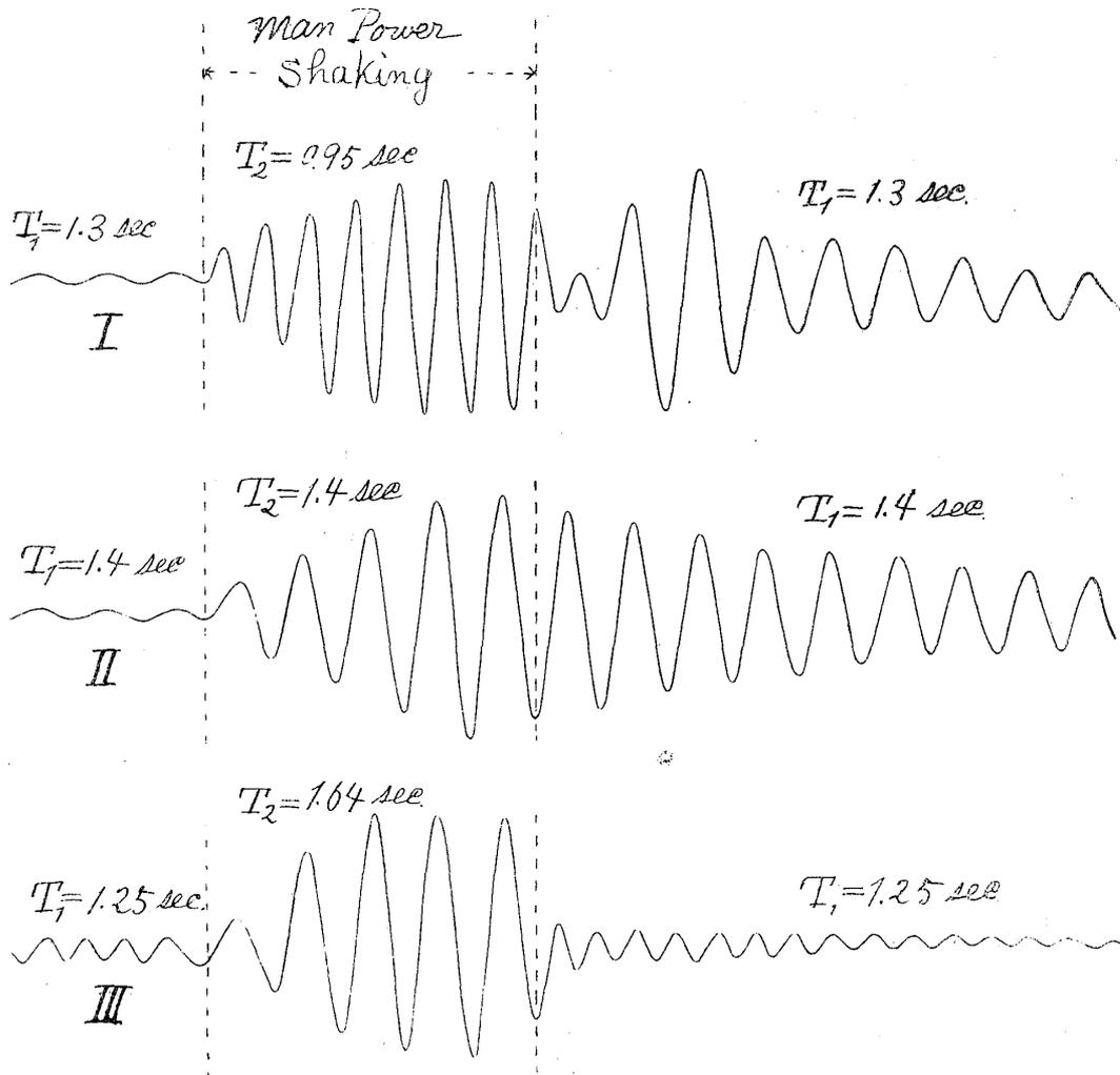
Fig. 14. Diagram illustrating the character of motion of the different gojunotos.
