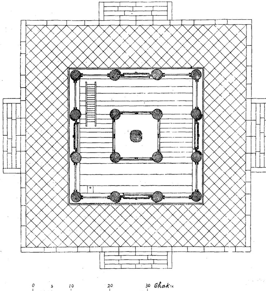
Fig. 2. Ground Plan of the Toji Gojunoto. (According to the drawing made by the late Mr. Y. Horiike. Scale in shaku (1 shaku=0.994 foot).
