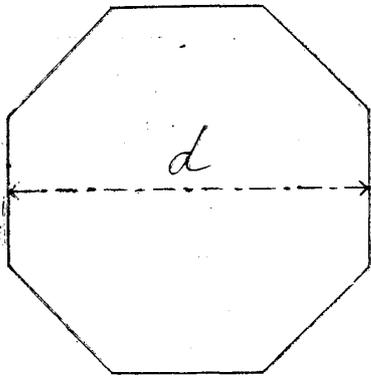
Fig. 11. Section of the Central Post of the Hommonji Gojunoto.
