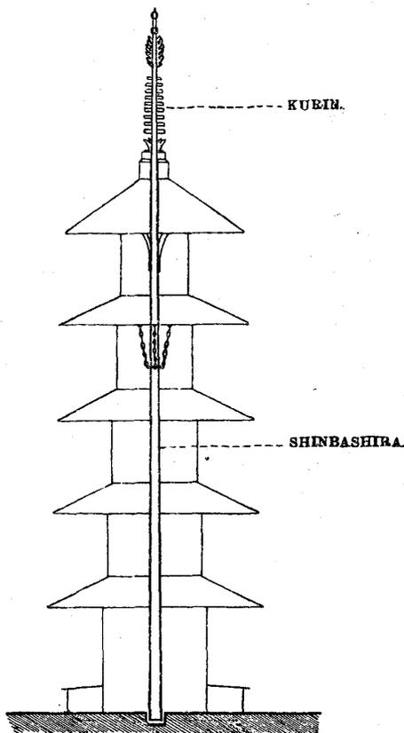
Fig. 1. Diagram showing the construction of Nikko Gojunoto.
