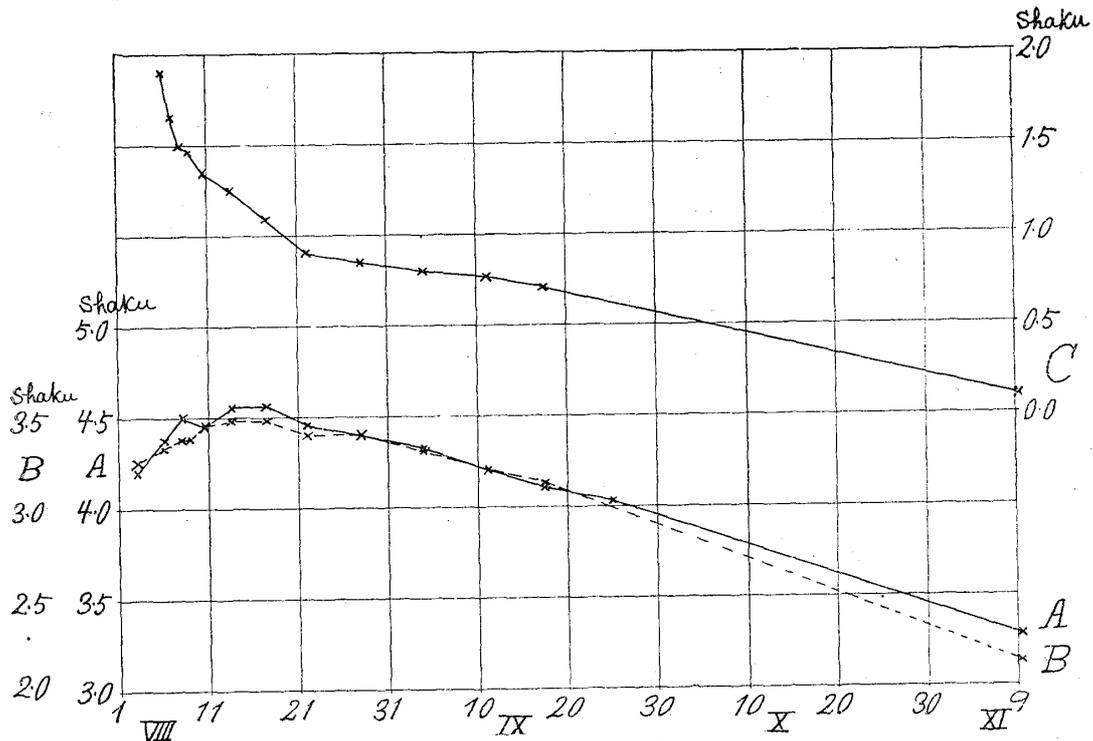
Fig. 11. Height Variation of the Surface of the Lake of Toya at different points of the Coast : Level Gauge Readings at the West Kohan School, Tokotan and Takinoue, Aug. 3rd to Nov. 11th, 1910.
