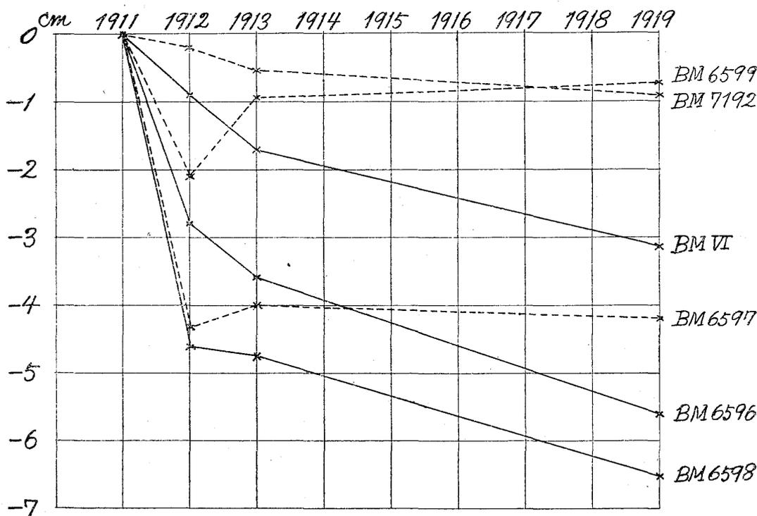
Fig. 2. Amount of the Height Change of the Different Bench Marks in 1912, and 1913, and 1919, referred to 1911.
