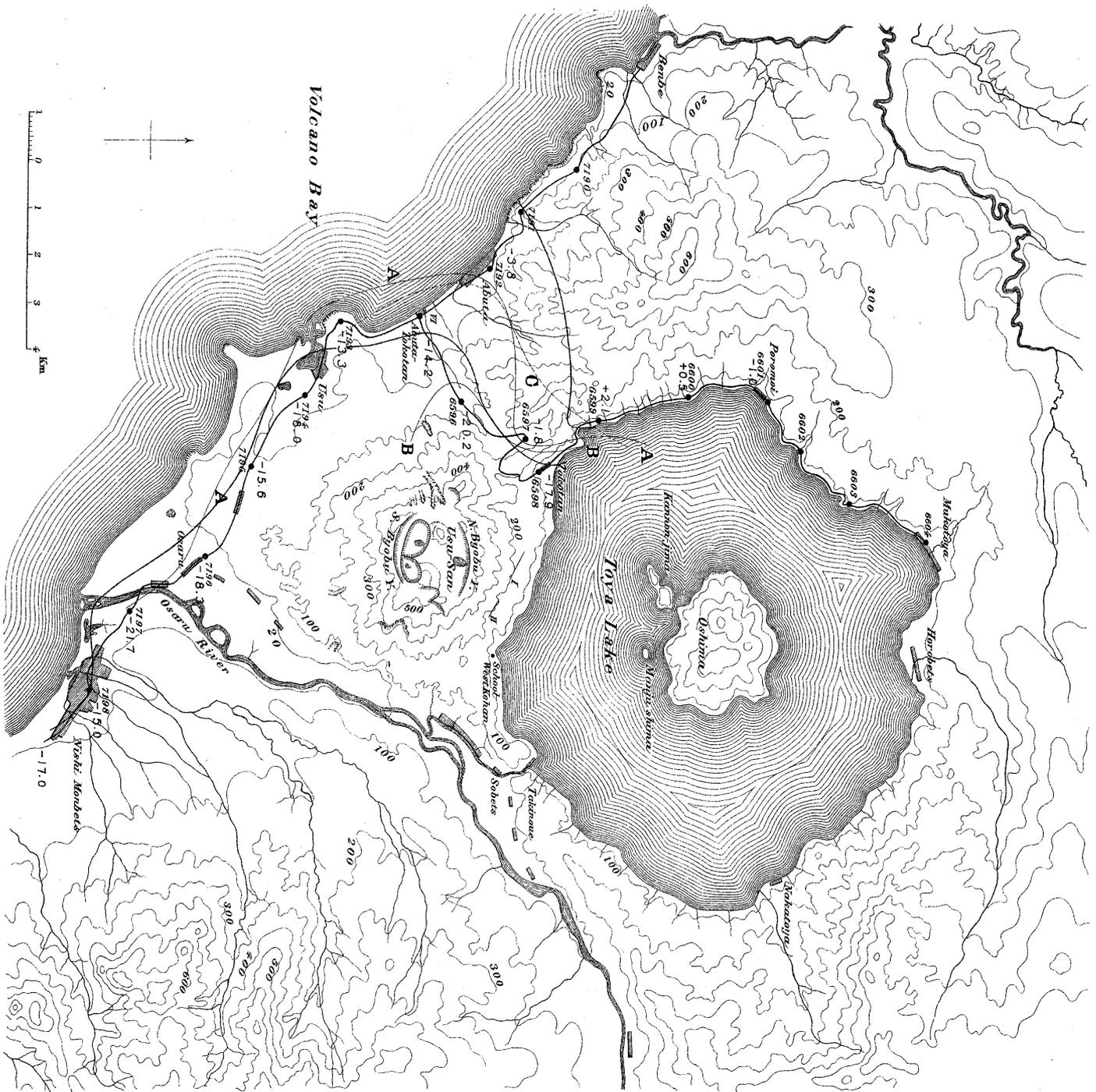
Fig. 3. Map showing the Height Difference in the Ust'-san District between 1913 and 1919, respectively 3 and 9 years after the Eruption. The outer (shorter) red curve is the line of no height change and the inner red curve is the line of 15 mm. depression of the ground in 1919 relative to 1913. The red figures indicate the change in the heights; plus (+) when augmented and minus (-) when lessened.
