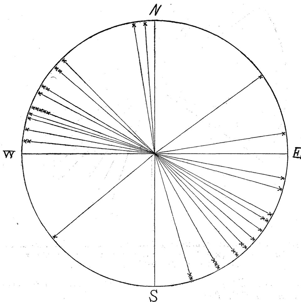
**Fig. 14. Diagram showing the Overturning Directions in the Northern Part of Kagoshima.**
