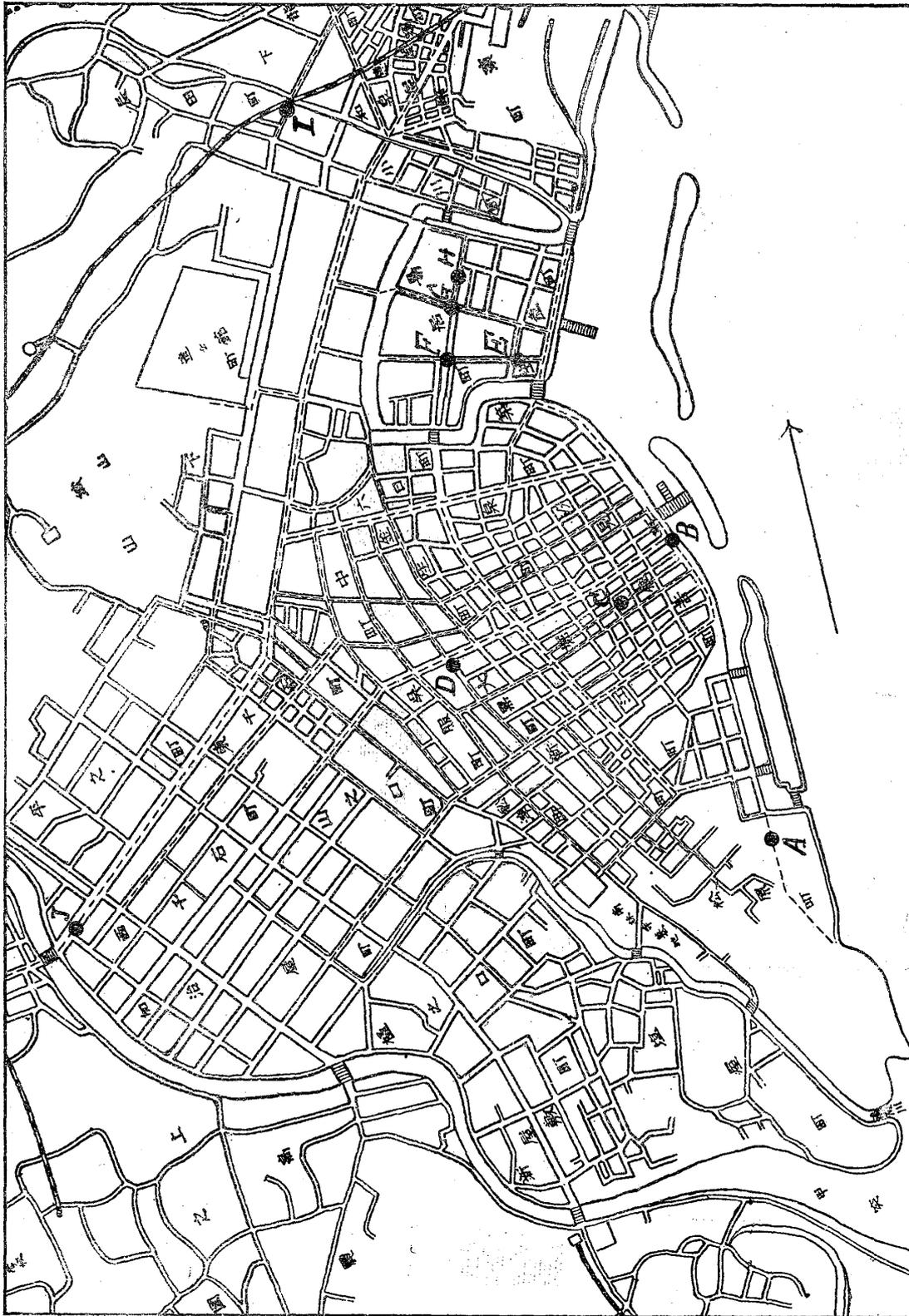
Fig. 24. Map of the City of Kagoshima, showing the Places (A, B, C,.....J) where the gas pipes were broken by the earthquake of Jan. 12, 1914. (Dotted lines indicate the location of the 2" to 8" gas pipes.)
