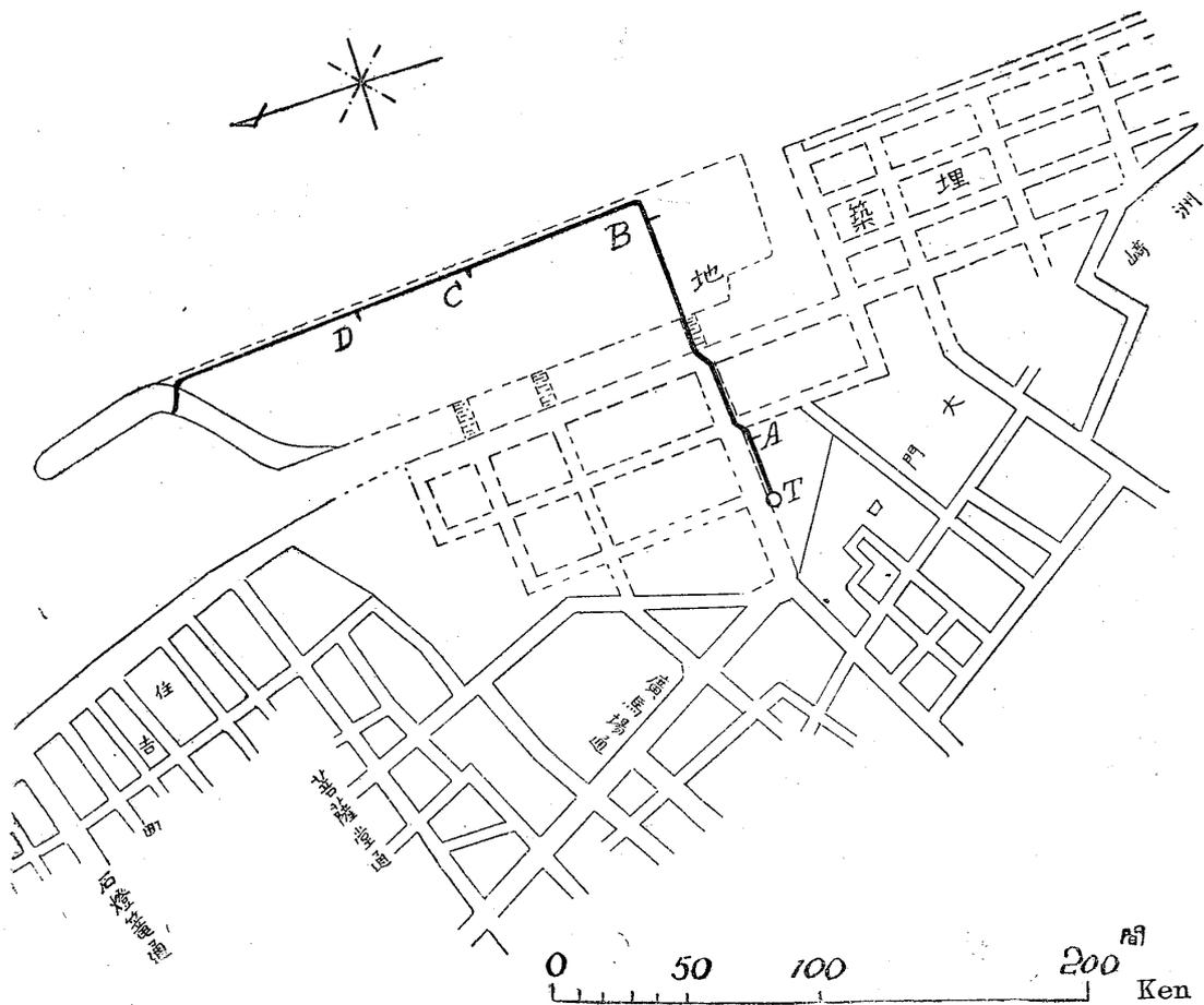
Fig. 21. Map showing the Location of the Oil Conducting Pipes (DBAT).
