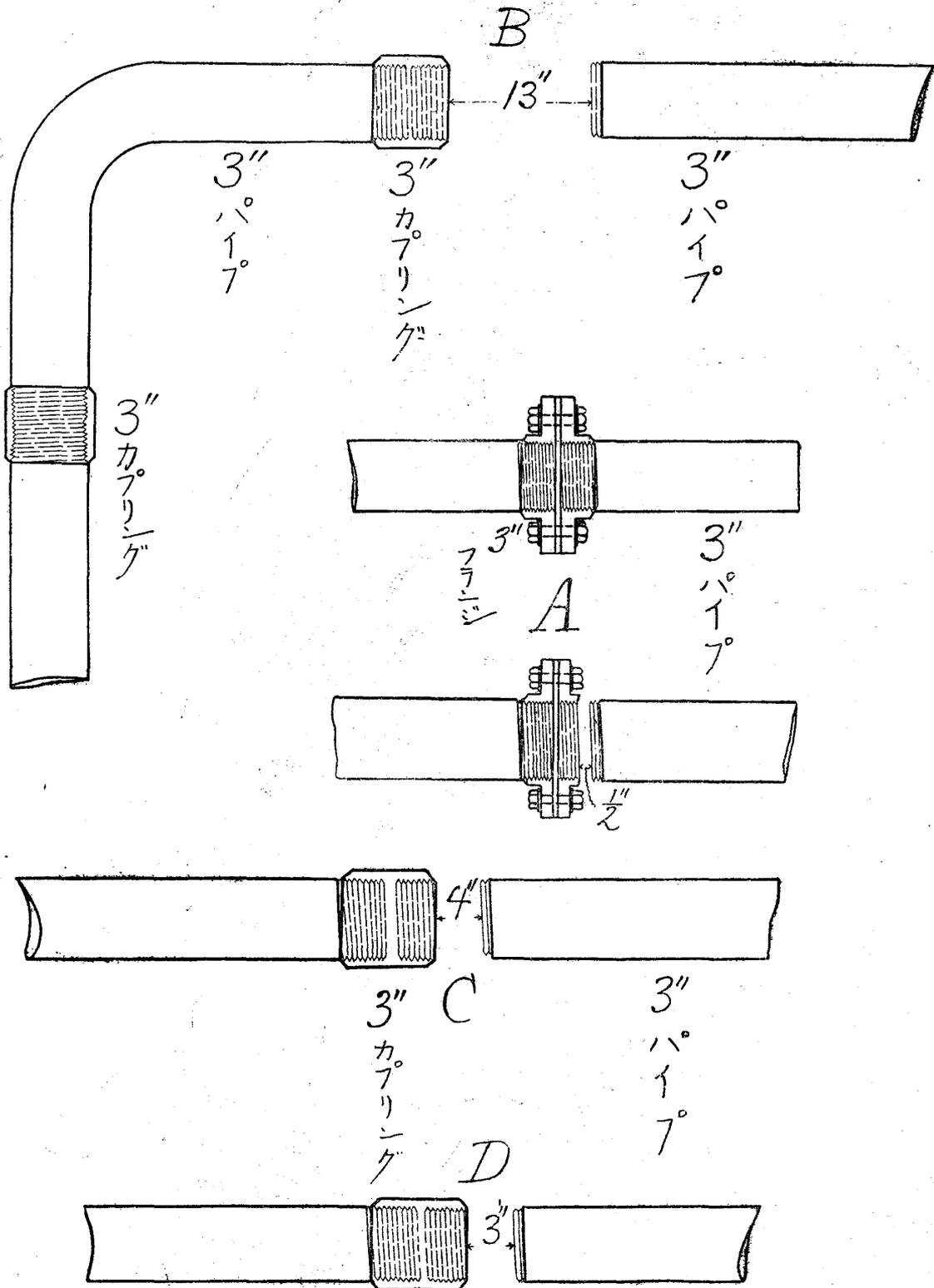
Fig. 23. Joint Fracture of the 3'' Oil Pipes.
