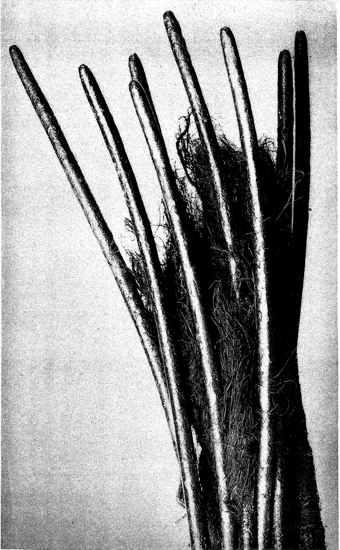
Fig. 33. An enlarged view of the Broken End of the 1" Telegraphic Cable between Kagoshima and Sakura-jima.
