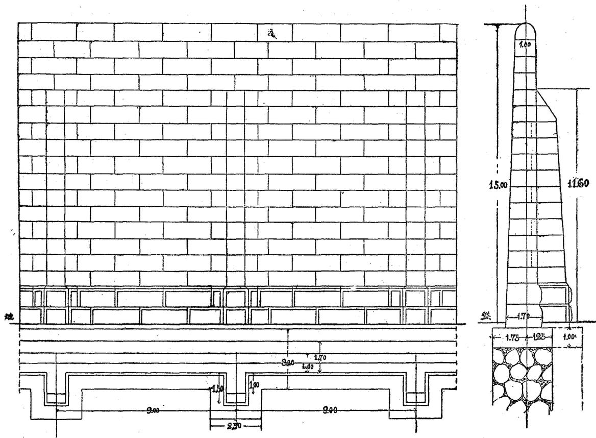
Fig. 16. Elevation, Plan, and Section of the Wall of the Kagoshima Prison.
