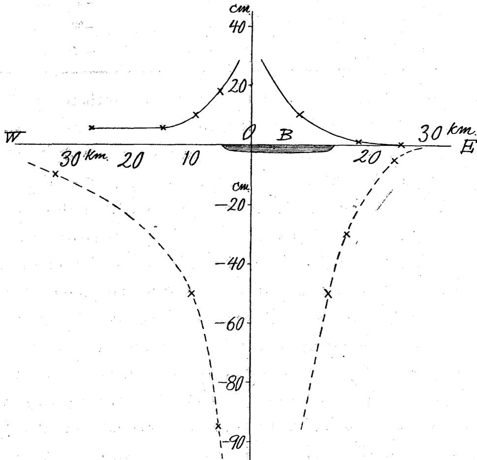
Fig. 3. Sectional Diagram representing the amount of the Depression caused by the Sakura-jima Eruption and of the subsequent Upheaval in an E.W. direction at varying radial distances from the Centre (0) of the Level Changes. The depression is measured downwards, and the elevation upwards, along the vertical axis drawn through 0.
