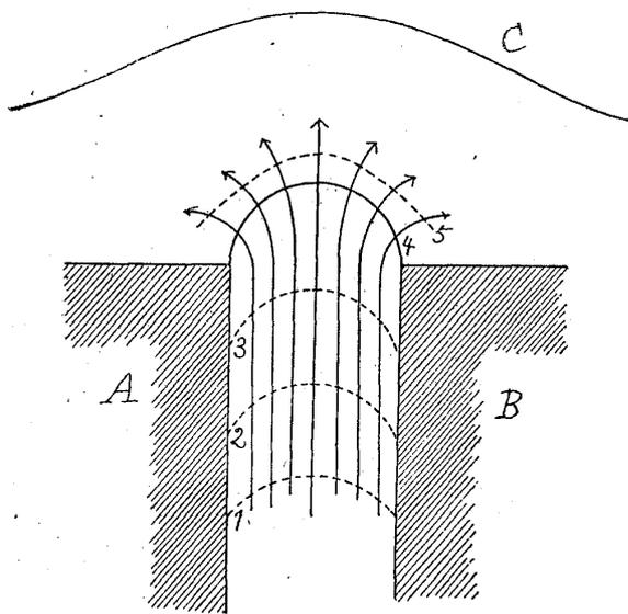
Fig. 32. Sectional Diagram illustrating the formation of an Internal Depression Cavity with Vaulted Roof.
