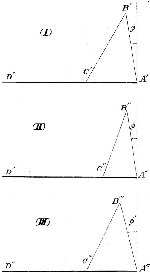
of the pendulum axis to the vertical, the ratios of multiplication  $\frac{A'C'}{C'D'}$  and  $\frac{A''C''}{C''D''}$  being unequal; while the two pendulums, I and III, have equal ratios of multiplication,  $\frac{A'C'}{C'D'}$  and  $\frac{A'''C'''}{C'''D'''}$ , but unequal angles of inclination of the pendulum axes,  $\phi$  and  $\phi'$ . The three pendulums are placed with their planes parallel to one another. Thus the first two pendulums would have an equal
