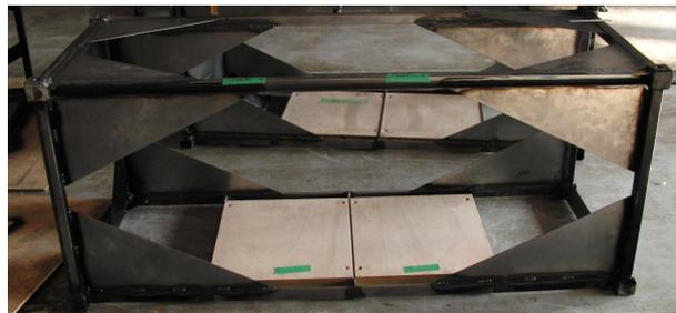
Figure 3.5: Constructed scaled model of a 20 ft container based on Froude scaling.
