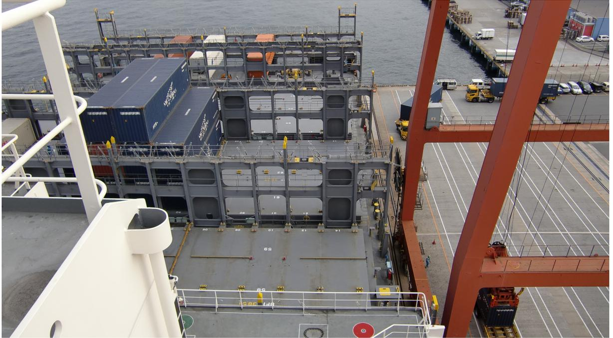
Figure 1.3: A picture taken from the deckhouse in the stern direction (NYK, THEMIS) during container loading procedure in Tokyo, Japan. The hatch and lashing bars can be clearly seen in the spots where additional containers still can be placed.
