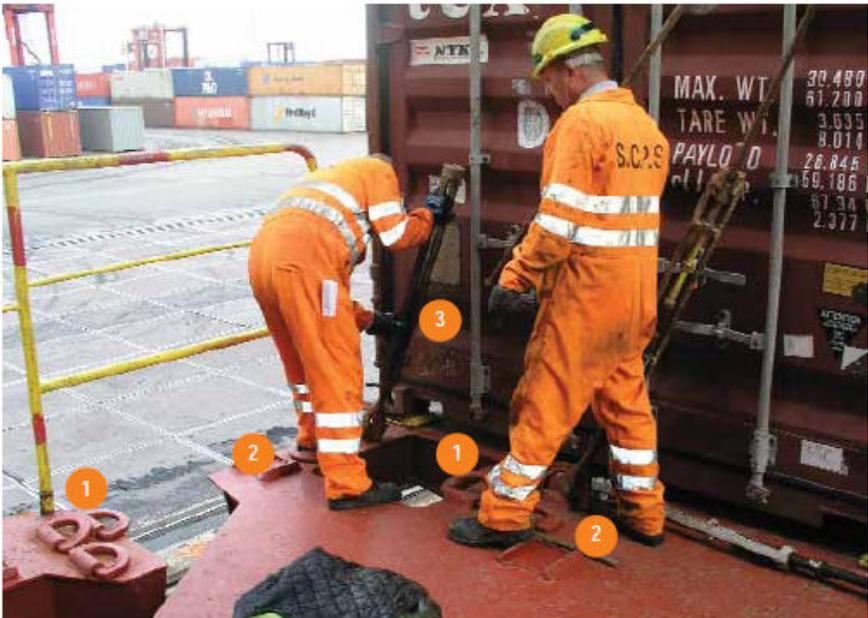
Figure 1.20: Lashing components being placed on a container ship [53].
