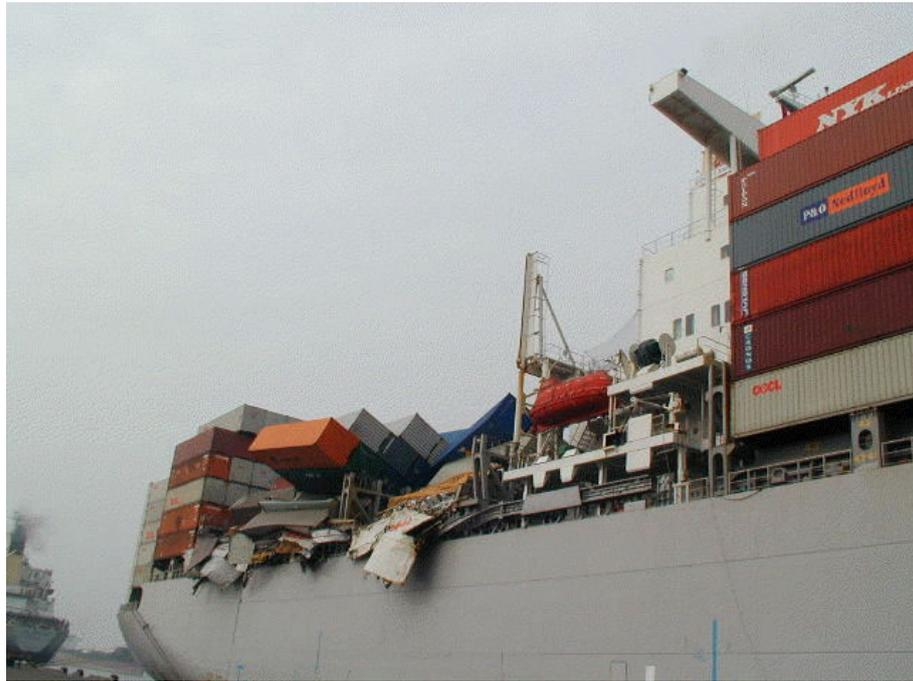
Figure 1.11: Another example of container stack collapse.
