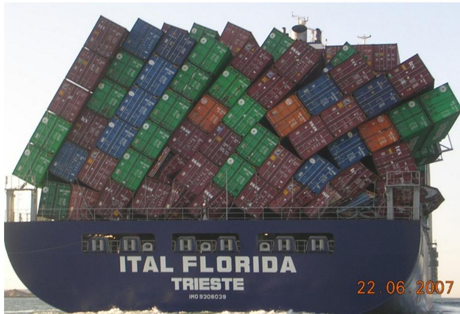
Figure 1.10: Total collapse of containers stacks with subsequent loss of top tiers.
