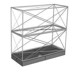
Figure 6.5: Finite element model of the two-tier single stack case (2x1).
