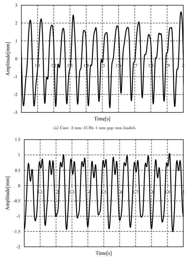
(b) Case: 2 mm–15 Hz–1 mm gap–loaded.
