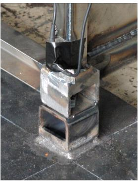
(b) Sockets were welded to the shaking table.
