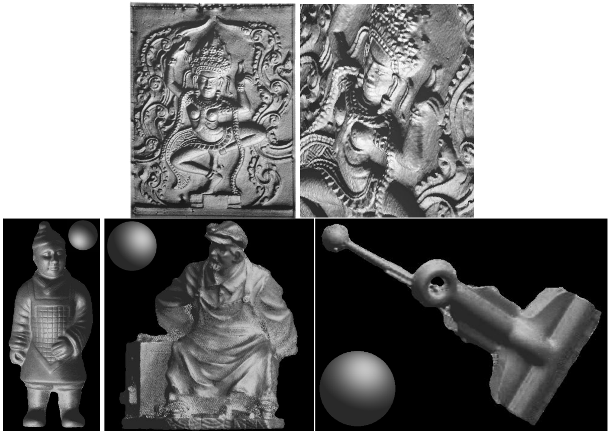
Figure 5.16: 3D reconstruction and relighting results. Top figures show 3D reconstruction of the relief scene from top view and close-up side view. Bottom figures show relighting results of terracotta, statue, and clip scenes. The reference spheres show rendering parameters.
