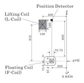
Figure 2.8: The schematic veiw of the arrangement of the F-coil, the L-coil and the position detectors.
