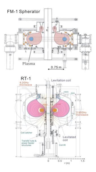
Figure 2.1: Comparison drawing of the magnetic field configurations of FM-1 Spherator and RT-1. Because the floating magnet in FM-1 Spherator was unstable to tilting direction, unlike that of RT-1, there're tilt stabilizing coils in FM-1 [after Ogawa (2009) [67]].
