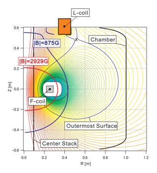
Figure 2.10: Magnetic field configuration of RT-1. When the F-coil is levitating: separatrix configuration. The magnetic field is stretched upward by the L-coil current.
