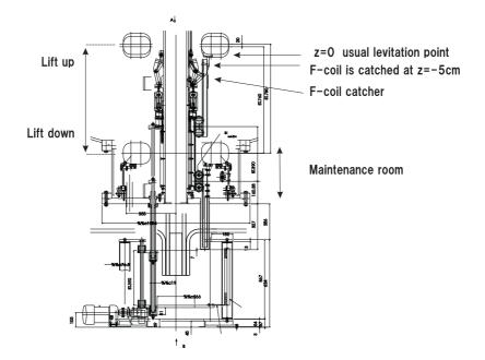
Figure 2.12: Schematic drawing of the RT-1 center stack structure. The mechanical lifter brings up and down the F-coil between the experiment room and maintenance chamber. The safety catcher can open within 0.1 second before the F-coil falls down 50 mm.
