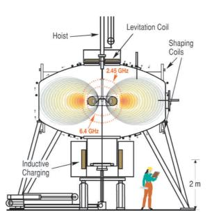
Figure 2.5: Schematic drawing of the LDX device [after Garnier (2006) [57]]. The camber radius is about 2.5 m and the volume of the plasma is designed large to obtain the stabilization effect of the plasma compressibility.
