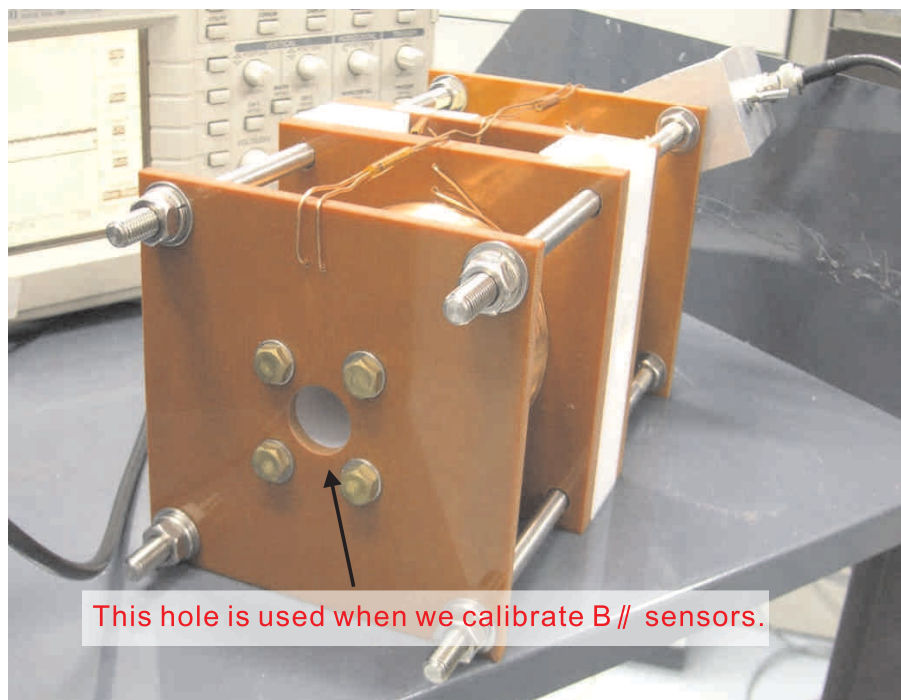
Figure 6.4: The photographs of the calibration coil. The coil is composed of a Helmholtz coil and is able to calibrate sensors in two directions, parallel and perpendicular to a probe axis.
