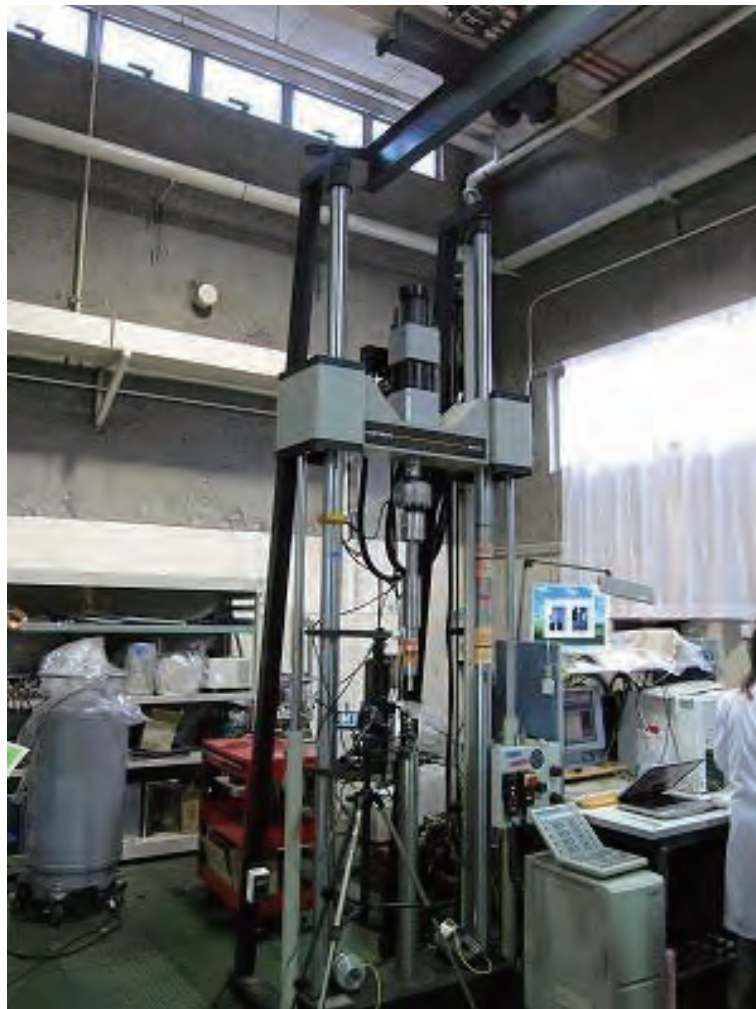
Figure 3.20: A fatigue-testing-system "INSTRON 8802" at NIMS
