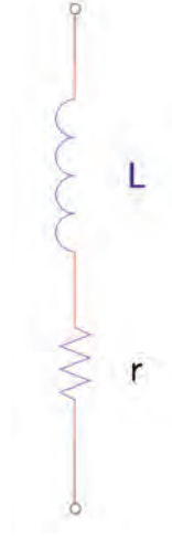
Figure 5.1: A circuit of a one turn coil with a FINEMET core
