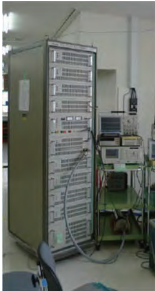
Figure 4.24: A semiconductor RF source
