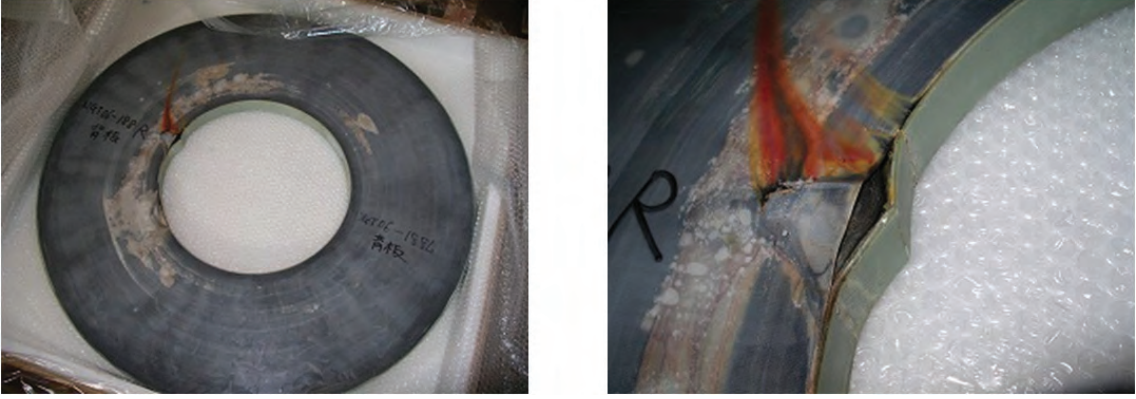
Figure 3.1: A picture of a buckled core (left). A closeup of the buckled area.
