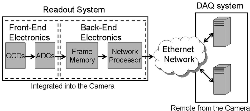
Fig. 1. Schematic diagram of the readout system, which consists of front-end electronics (FEE) and back-end electronics (BEE). The FEE reads data from the CCDs and digitizes these data. The BEE stores the digitized data and transfers these data to a DAQ system. The DAQ system analyzes these data as images.
