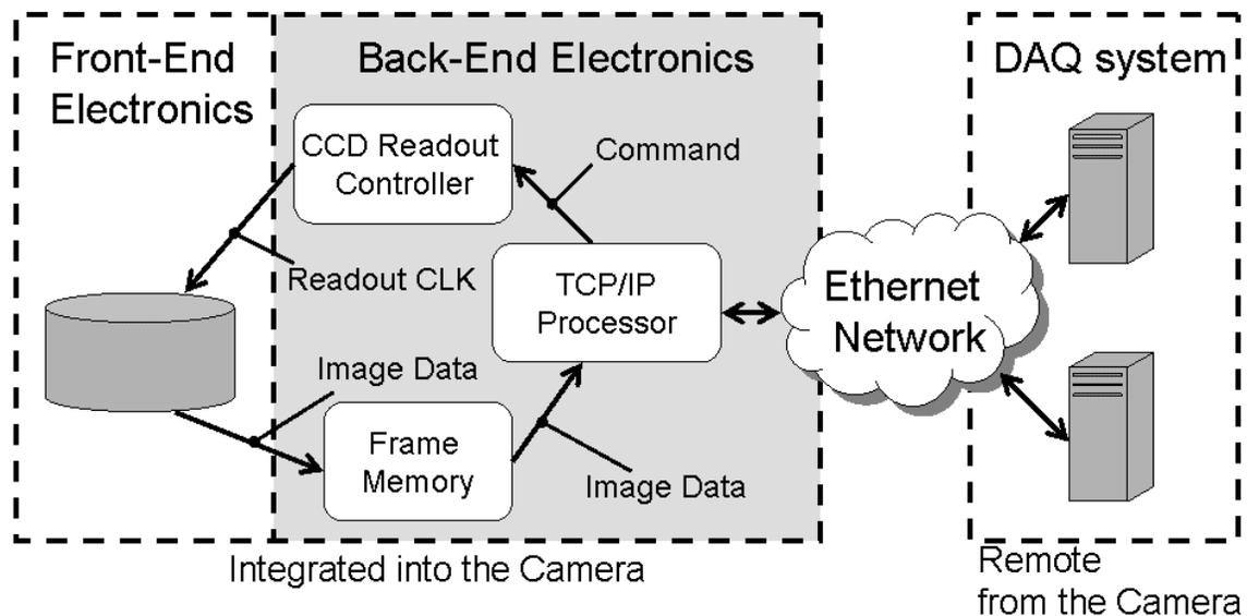
Fig. 2. Schematic of the readout system.
