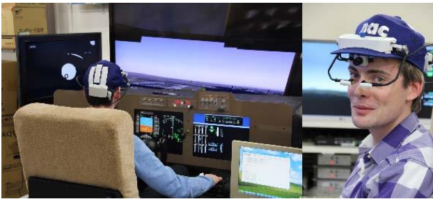
Fig. 5 The NAC EMR-8 eye-mark recorder.
